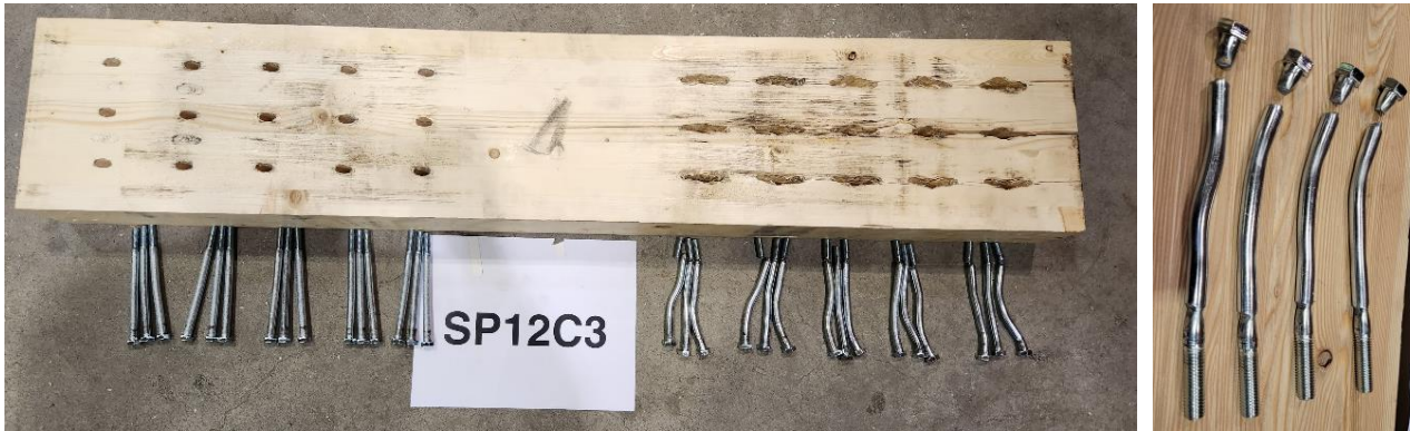
Figure 5. Typical wood crushing followed by splitting of a typical brace with non-reinforced connections (left) (15 d_F=9.5\text{mm} bolts; S_p=9.4d_F ); Bolt rupture in the shank near the head (right).
