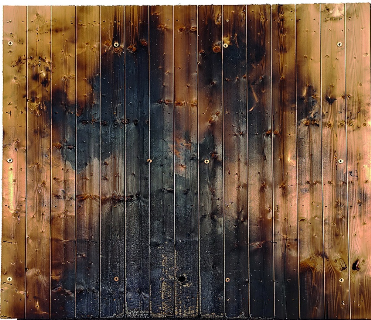
Figure 7: Photo documentation of the wooden cladding above the fire stop after completion of the test and the observation time for test 3
