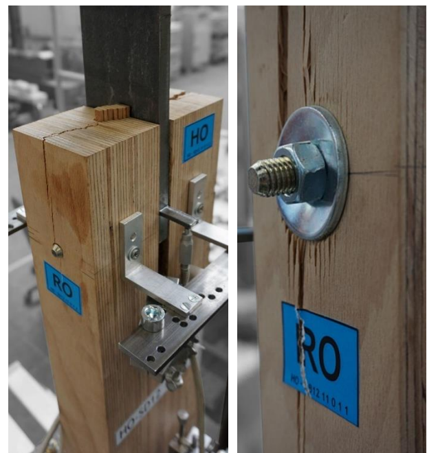
Figure 3.2. Splitting of the timber after ductile deformation of the dowel and deformation of a bolt and the washer ( \alpha = 0^\circ )
