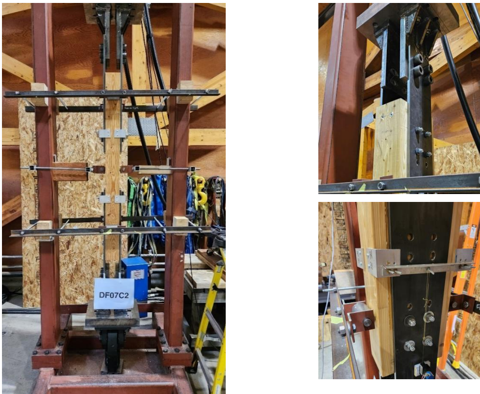
Figure 3. The test setup with a brace specimen ready for testing (left); Example of a top reinforced connection (top right) and a bottom unreinforced connection (bottom right)
