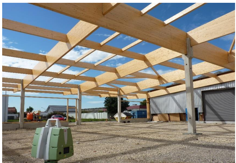
Figure 1.1. On-site imperfection measurement with a laser scanner Leica ScanStation P20 (building 2020-KW34).
