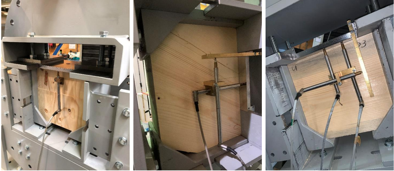
Figure 2.2. Applied devices for way measurement in case of axial (left), lateral (middle) and combined loading (right)
