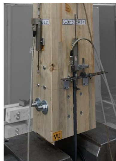
Figure 1.1. Tensile test on steel-timber connection with 2x3 fasteners
