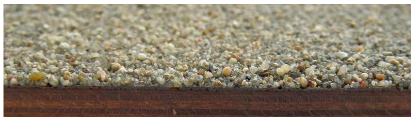
Figure 10. Coated surface with 2K epoxy resin and quartz sand 0-2 mm.
