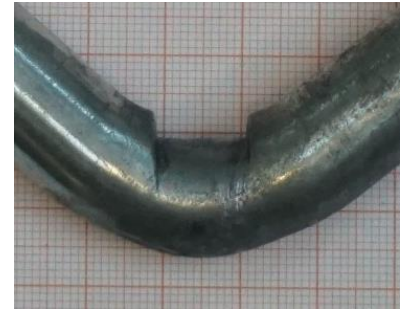
Figure 3.2. Occuring plastic deformations of the fastener for large bending angles
