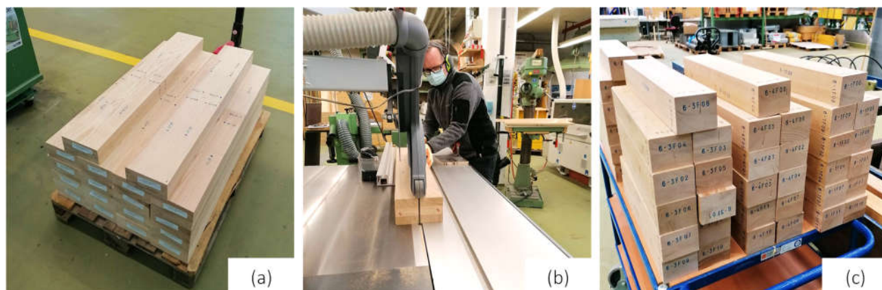
Figure 2: In order to receive almost identical specimens (with regard to density, annual ring width, etc.) in all climatic conditions, glulam and LVL elements were labeled (a) and then cut into half in the longitudinal (b) and transversal direction (c).
