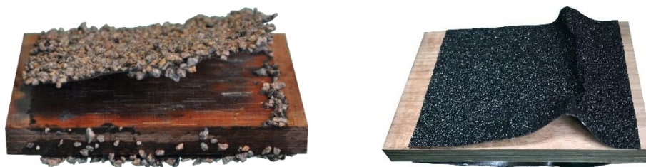
Figure 16. Coated test specimens: 2K adhesive and grit (left) and griptape (right).
