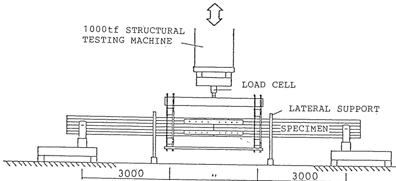
Fig.2 BENDING TEST APPARATUS
