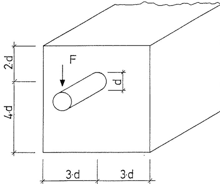
Fig.3: Minimum edge distances to avoid perpendicular-to-grain tension failures
