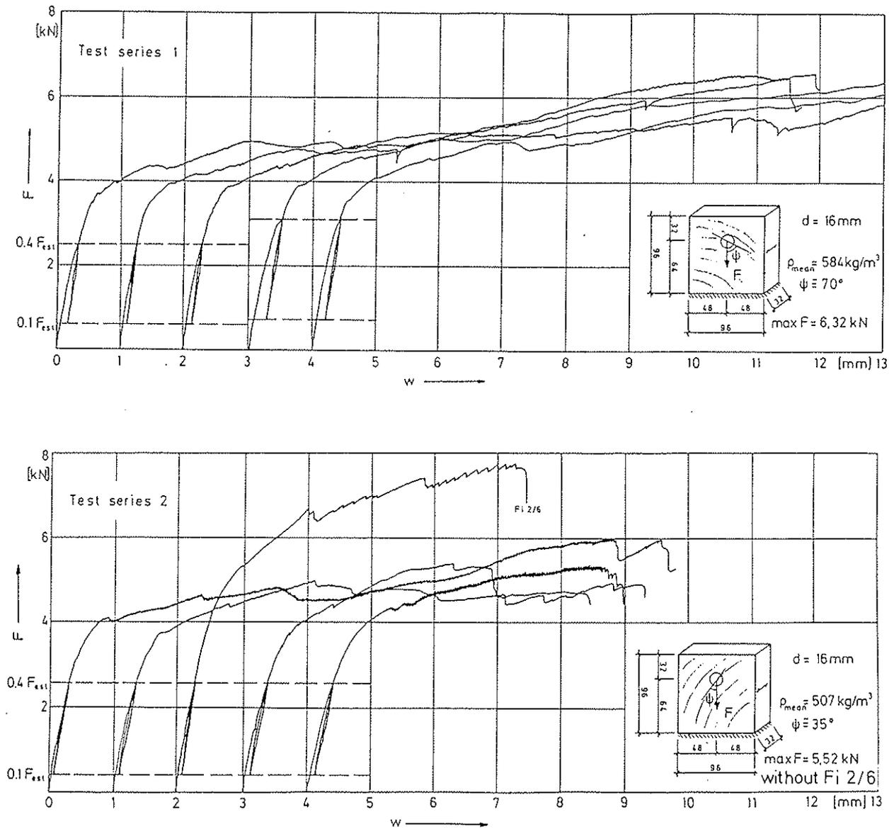
**Fig.6:** Load-deformation curve of specimens with a dowel-type fastener loaded in compression perpendicular to grain in a prebored hole parallel to grain
