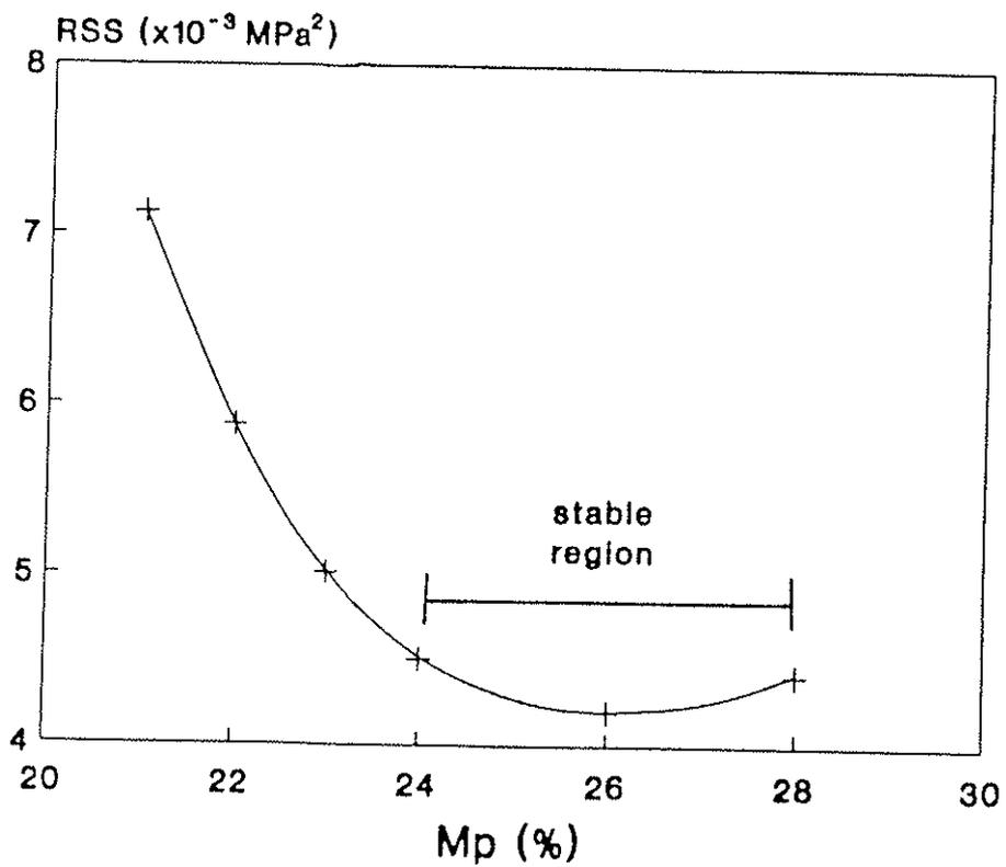
Figure 7: Relationship between the Intersection Moisture Content ( $M_p$ ) and the Residual Sums of Squares (RSS) for the general 2-term MOR Linear Surface Model (Douglas-fir)
