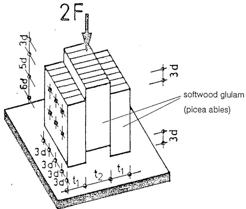
Fig. 1: Test specimen and dimensions;
