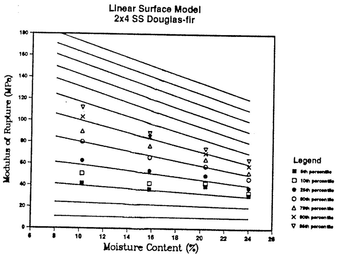
Figure 11: Predicted Modulus of Rupture Using 4-Term Linear Surface Model
