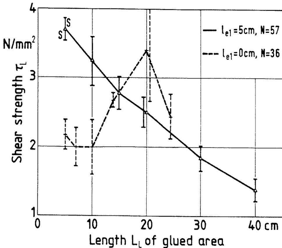
Figure 6: Effect of length  $L_L$  of glued area
