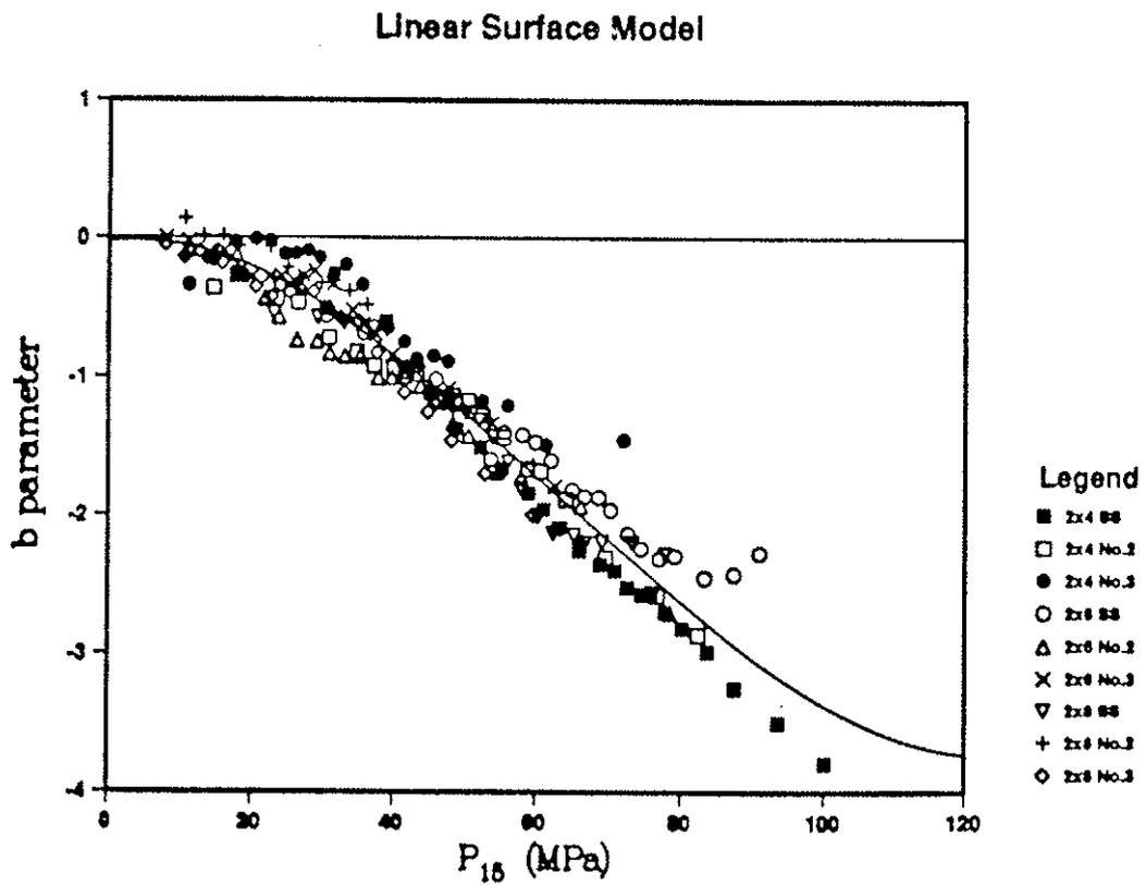
Figure 8: Relationship between the  $b$  parameter and  $P_{15}$  for 4-Term Linear Surface Model and showing the cubic regression fit to Douglas-fir *MOR* data
