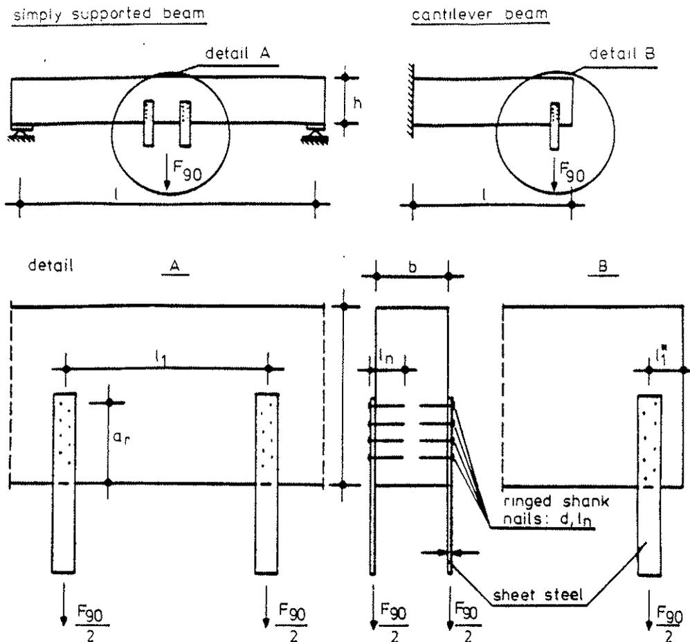
Fig. 3: Test set-up for steel-to-wood joints loaded perpendicular to grain (Ehlbeck / Görlacher [4]).
