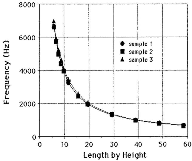
Figure 5. Effect of length by height of specimen on measuring fundamental vibration frequency
