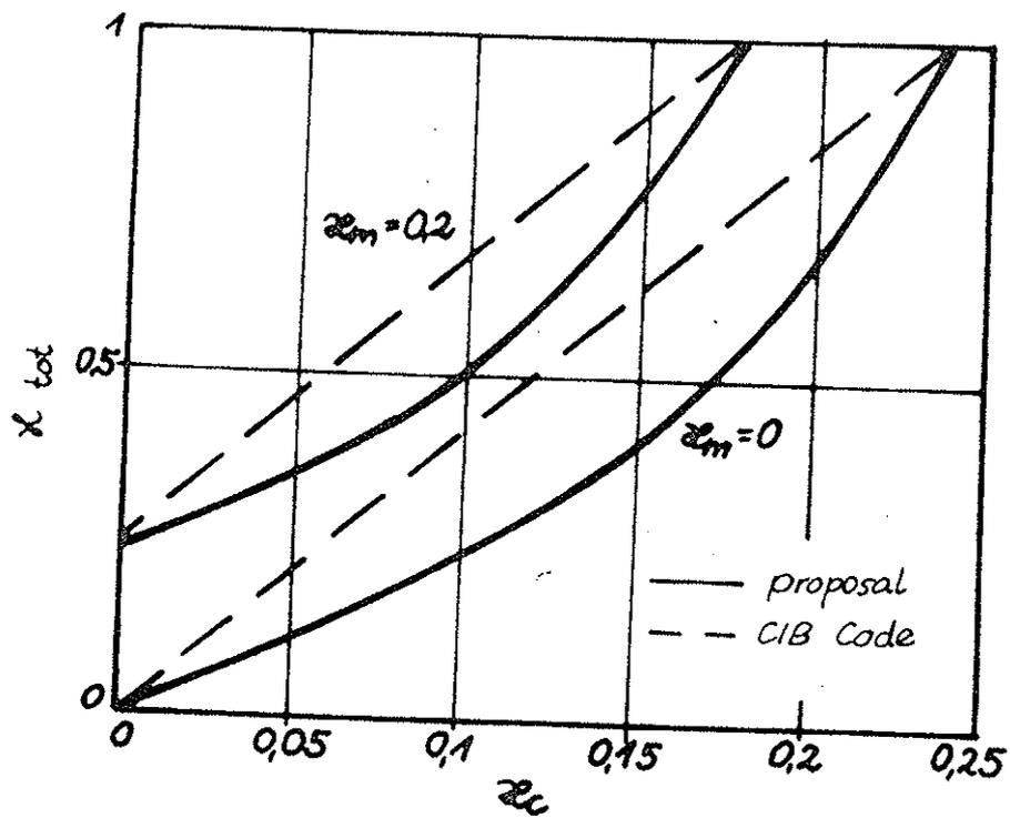
Figure 4: Comparison in terms of the components of  $X_c$  and  $X_m$  in  $X_{tot}$  for  $\lambda = 100$
