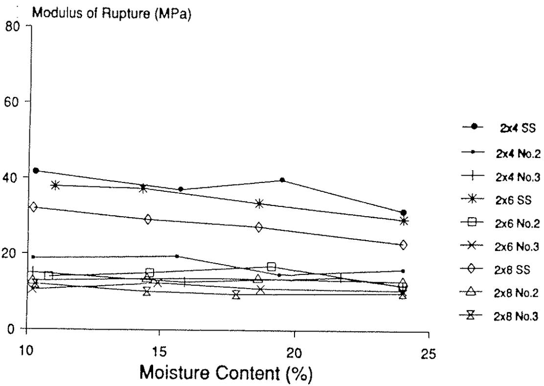
Figure 1: Relationships between the fifth percentile modulus of rupture and moisture content for Douglas-fir ( $M_p = 24$ ) (Aplin *et al* 1986)
