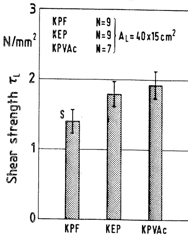
Figure 11: Effect of glue type on shear strength  $\tau_L$
