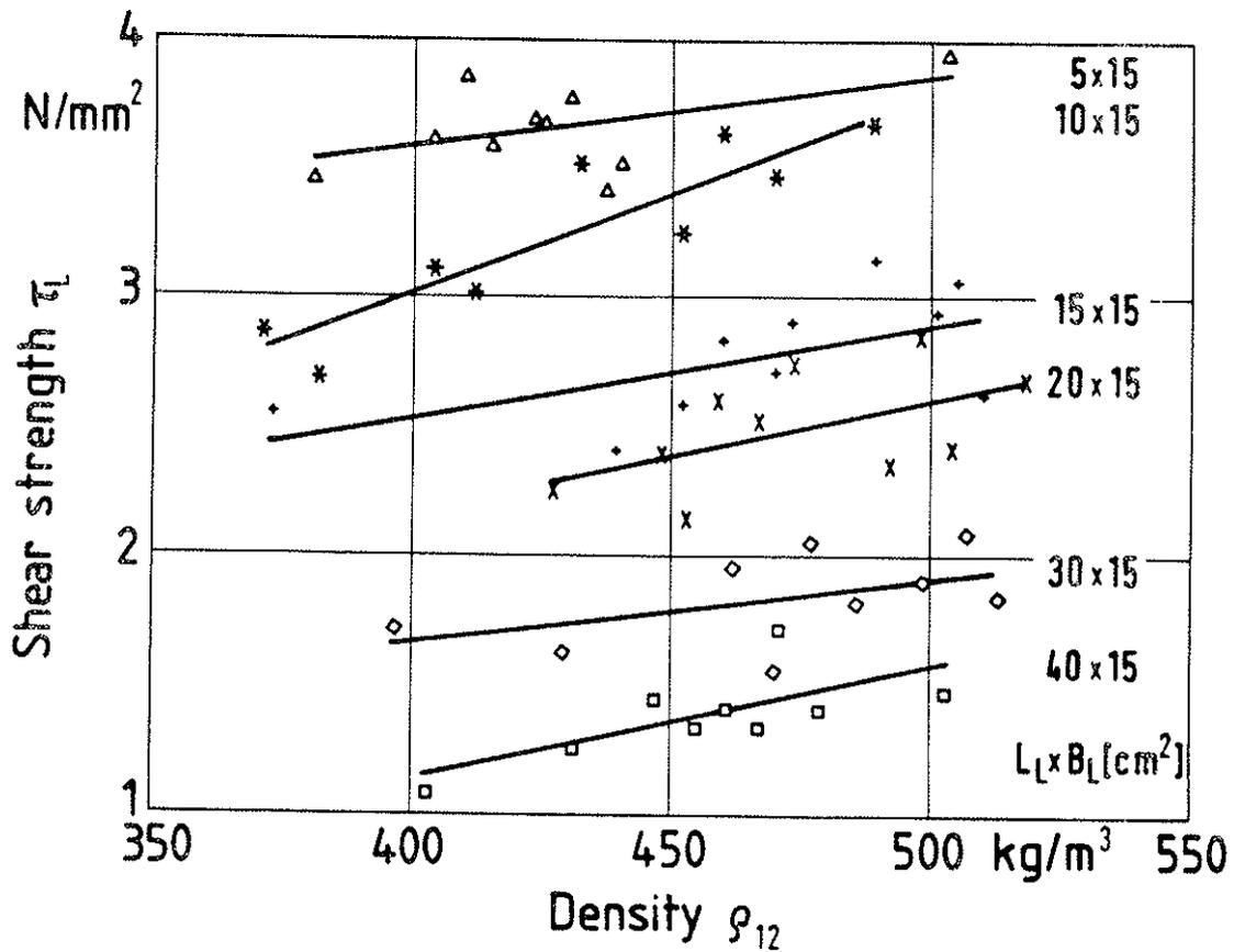
Figure 12: Effect of density  $\rho_{12}$  on shear strength  $\tau_L$  for different sizes of glued area ( $A = L_L \cdot B_L$ ,  $\alpha = 0^\circ$ ,  $l_{e1} = 5$  cm)
