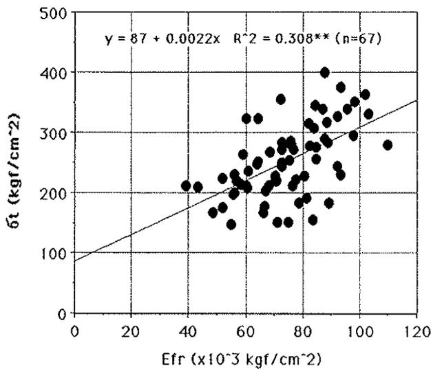
Figure 3. Relationship between Efr and tensile strength ( $\sigma_t$ )
