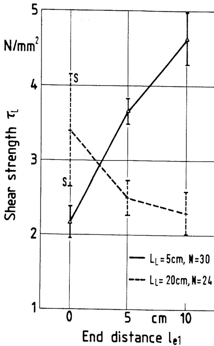
Figure 4: Effect of end distance  $l_{e1}$  on shear strength  $\tau_L$  for specimens with different lengths of glued area ( $L_L = 5\text{ cm}, L_L = 20\text{ cm}, \alpha = 0^\circ$ )
