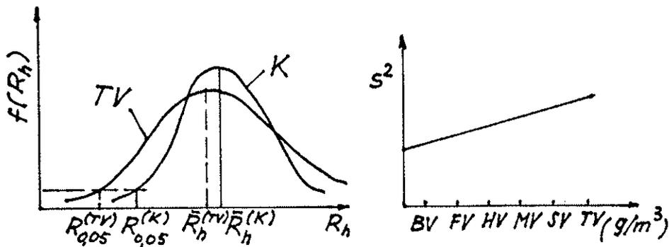
In the case of the specimens saturated with preservative the standard deviation and coefficient of variation are increasing hence the values of  $R_{0.05}$  and  $R_{0.001}$  (5 per cent and 0.1 per cent exclusion limit respectively) are decreasing. The figures that follow indicate the general feature of the tensile strength data obtained for specimens of *Picea excelsa* ("K"-control specimens, "TV"-preservative-treated material).
