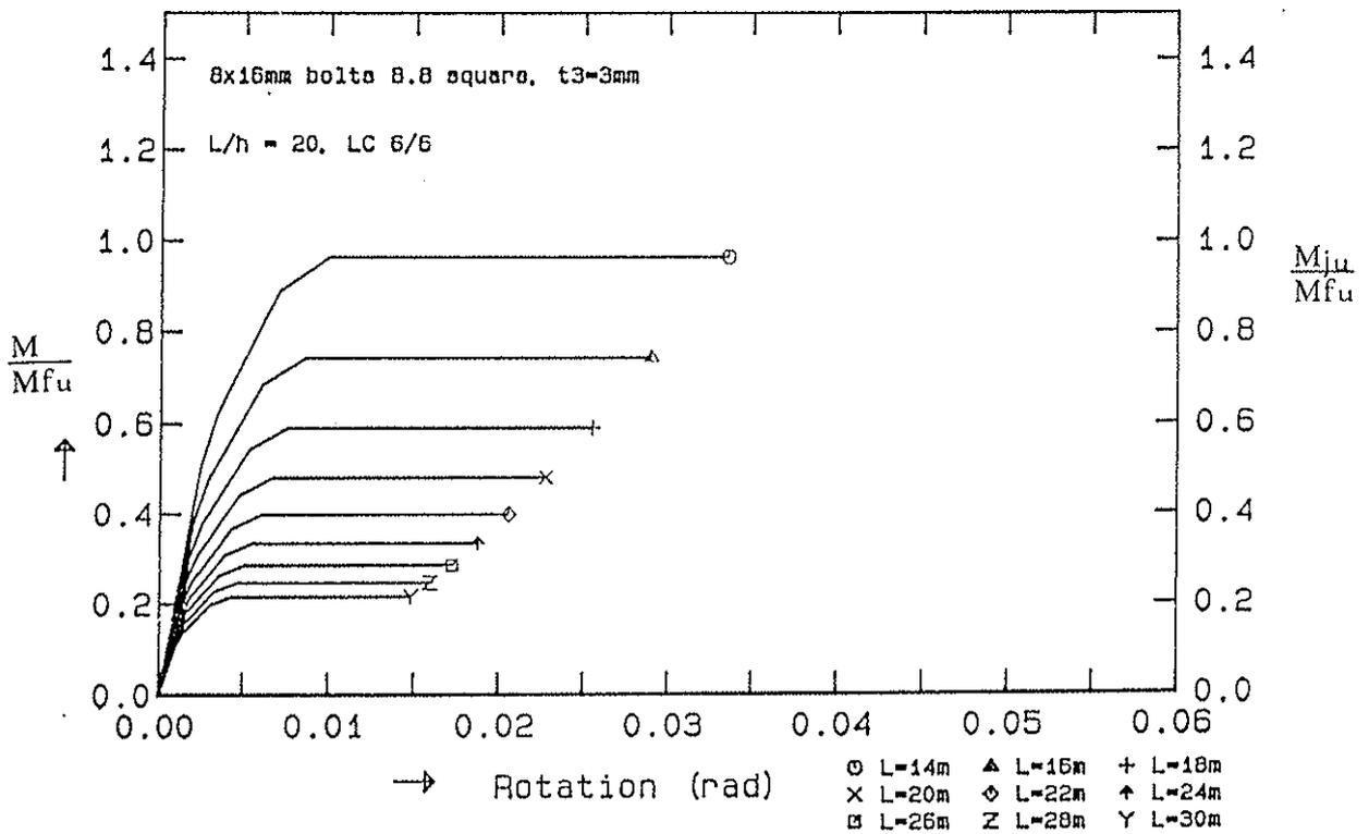
fig.9: Moment rotation curves of a steel reinforced joint with a square pattern
