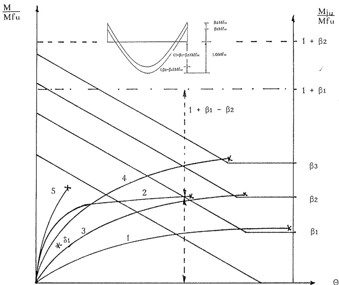
fig.7: Moment-rotation requirements combined with several moment-rotation curves.
