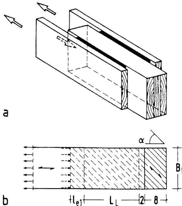
Figure 2: Specimen for basic joint tests
