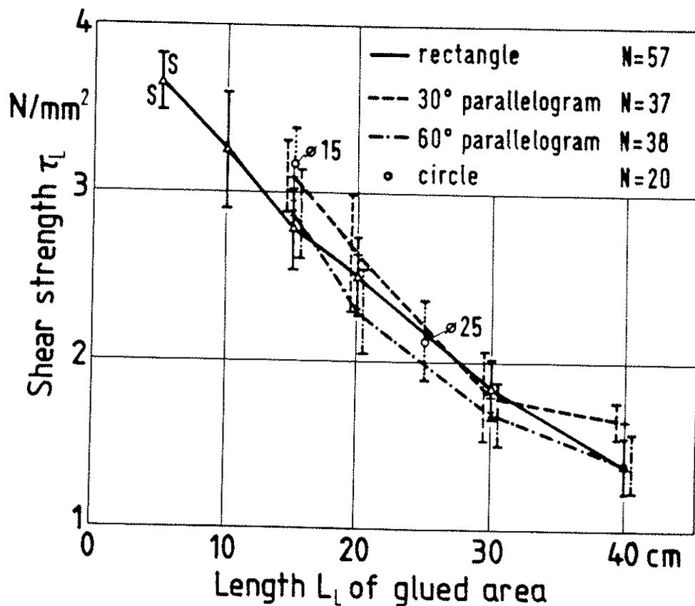
Figure 8: Effect of shape of glued area on shear strength  $\tau_L$  for different lengths of glued area ( $l_{e1} = 5$  cm,  $\alpha = 0^\circ$ )
