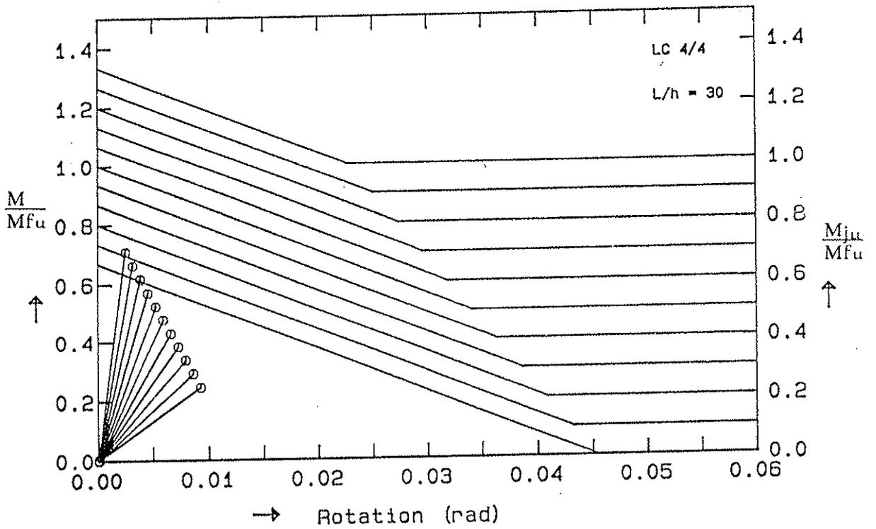
fig.4: Normalized moment - rotation graph with  $\beta$  increments of 0.1
