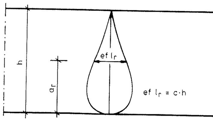
Fig. 7: Assumption for  $ef l_r$  in case of one fastener per row, only
