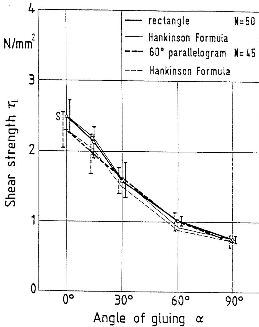
Figure 9: Effect of angle of gluing  $\alpha$  on shear strength  $\tau_L$
