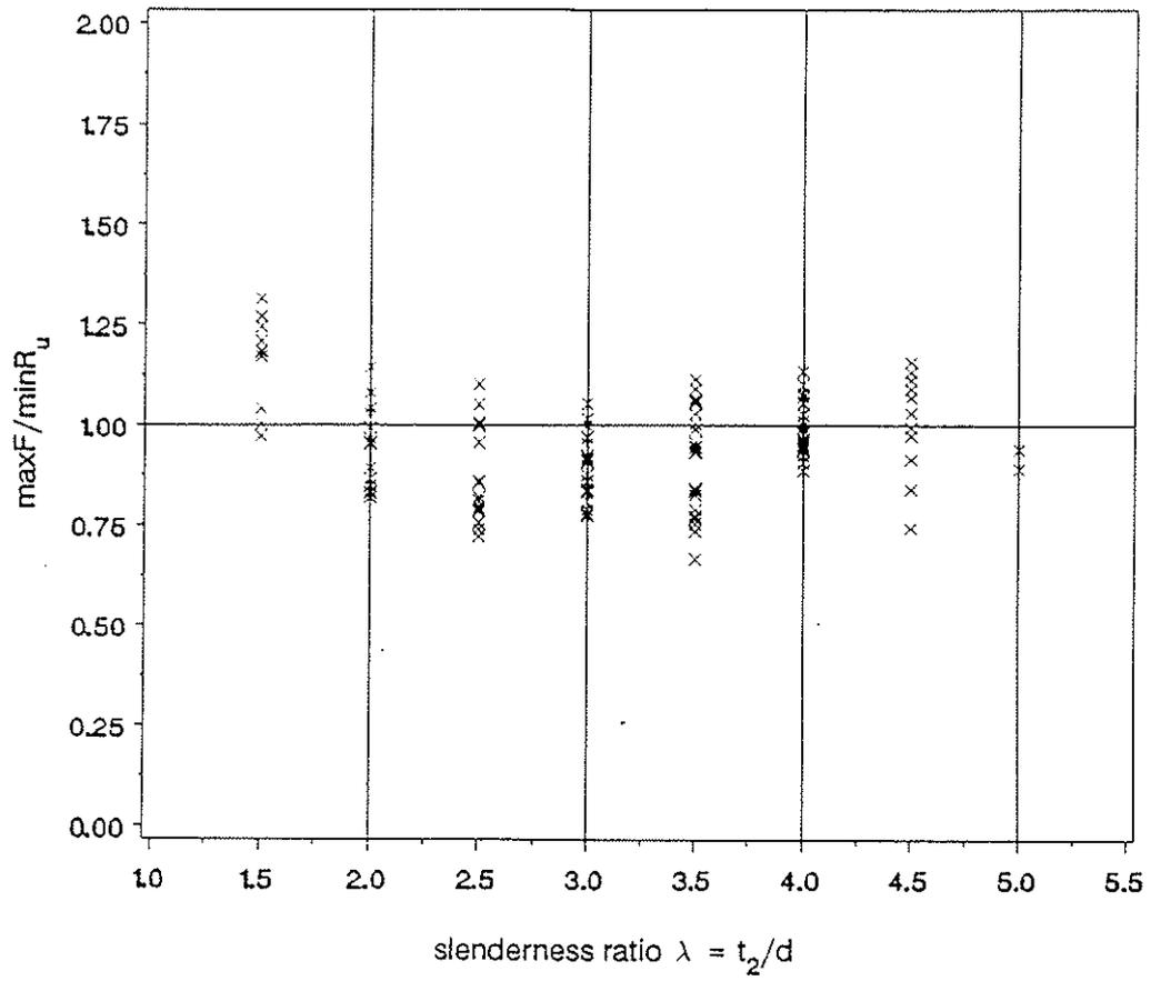
Fig. 5: Ratio  $\max F / \min R_u$  over slenderness  $\lambda$  for all tests
