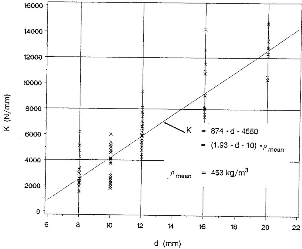
Fig. 7: Slip modulus  $K$  over dowel diameter, achieved from tests and evaluated according to ISO 6891 (128 test values)
