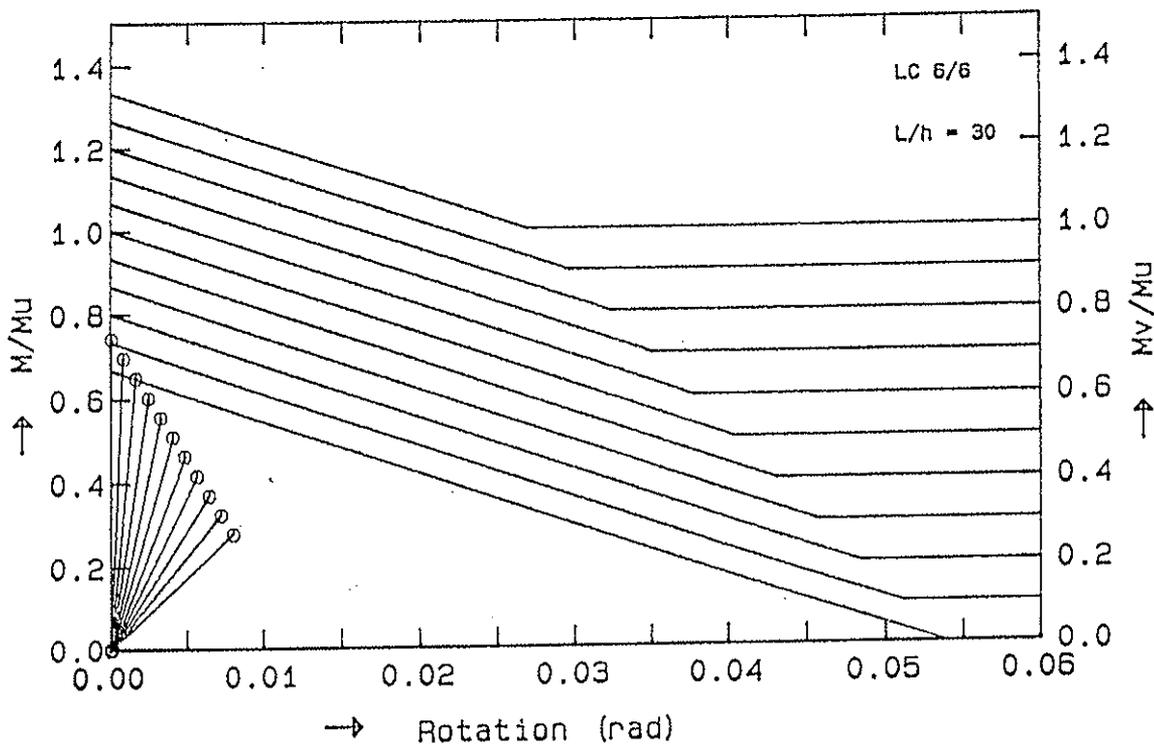
fig.5.: Normalized moment - rotation graph with  $\beta$  increments of 0.1
