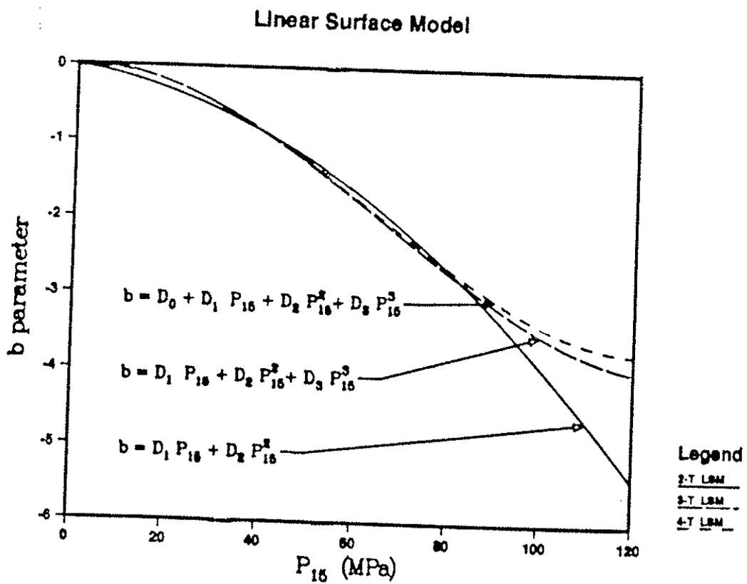
Figure 9: Regression fits of  $b$  parameter for the 4-, 3-, and 2-Term Linear Surface Models for the MOR data
