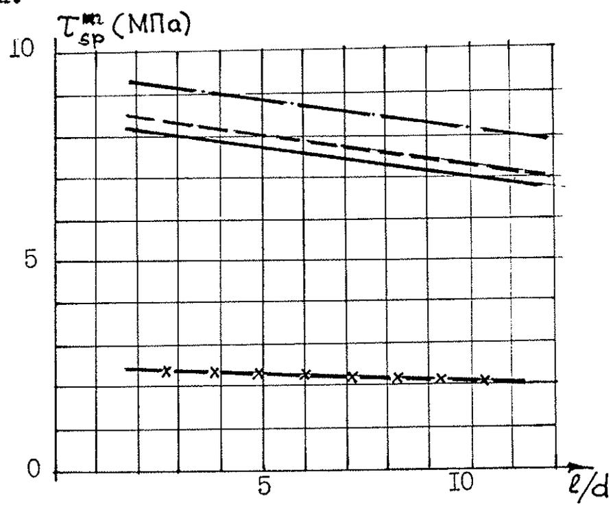
Fig. 2. Relationship graph for average spalling stress  $\tau_{sp}^m$  of  $1/d$ .
