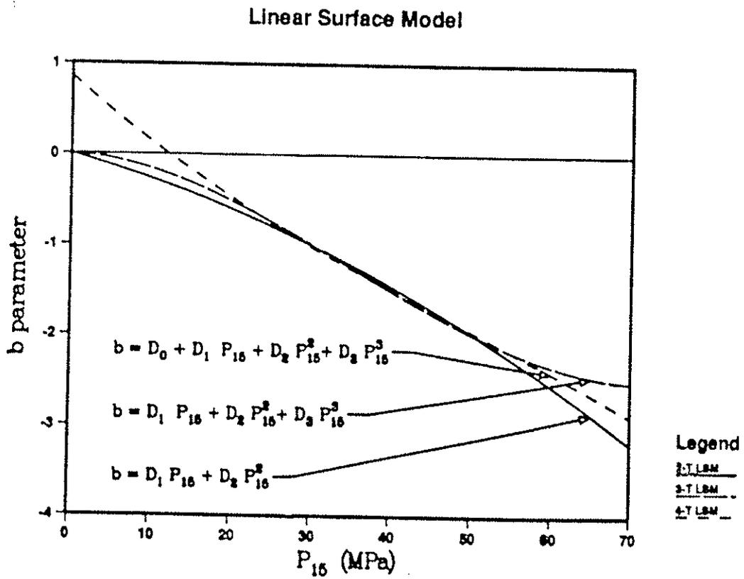
Figure 13: Regression fits of  $b$  parameter for the 4-, 3-, and 2-Term Linear Surface Models for the compression strength data
