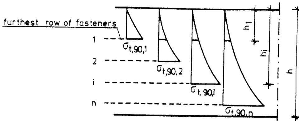
Fig. 6: Distribution of tensile stresses perpendicular to grain, generated in  $n$  rows by the load  $F_{t,90,n}$ .
