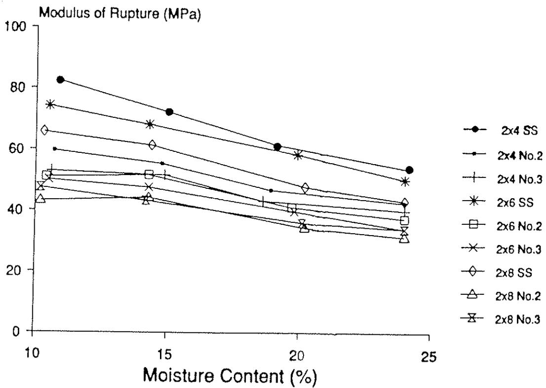
Figure 3: Relationships between the fifth percentile modulus of rupture and moisture content for southern pine ( $M_p = 24$ ) (McLain *et al* 1984)
