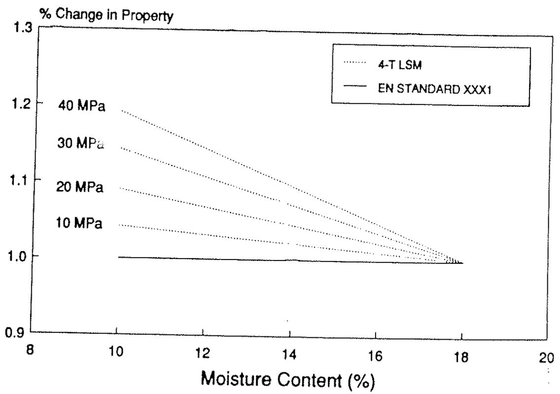
Figure 20: Comparison between CEN recommendations and 4-term MOR linear surface model
