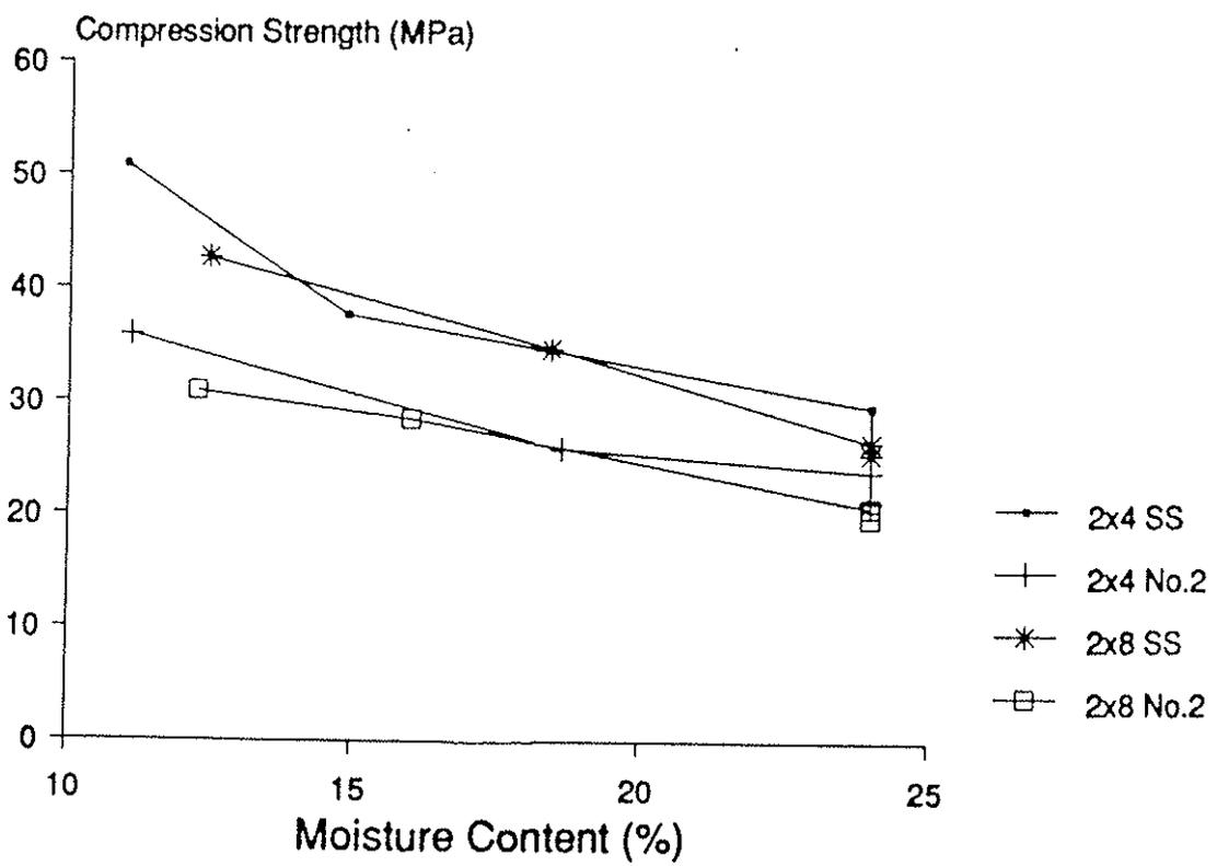
Figure 5: Relationships between the fifth percentile compression strength and moisture content for Douglas-fir ( $M_p = 24$ )
