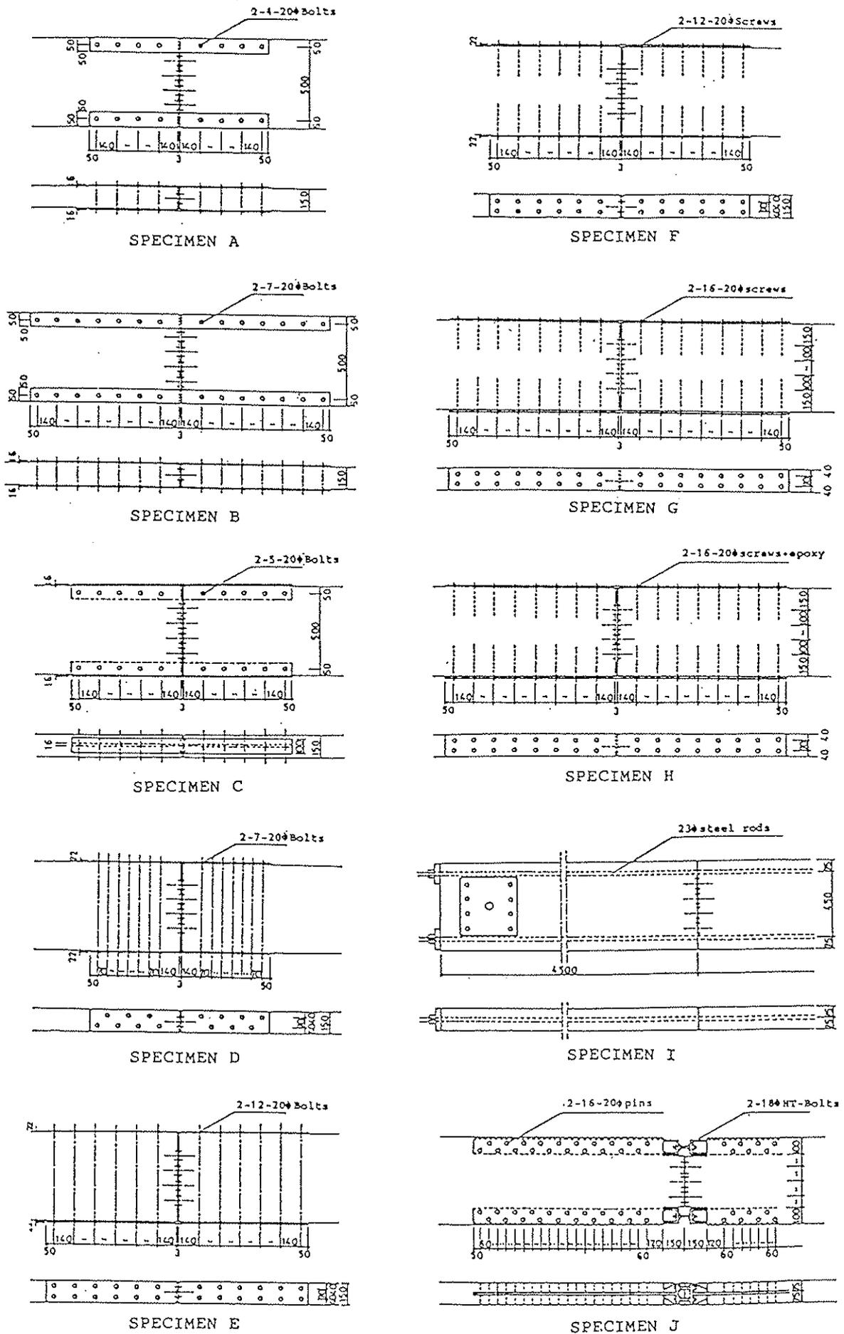
Fig.1 DETAILS OF SPECIMENS
