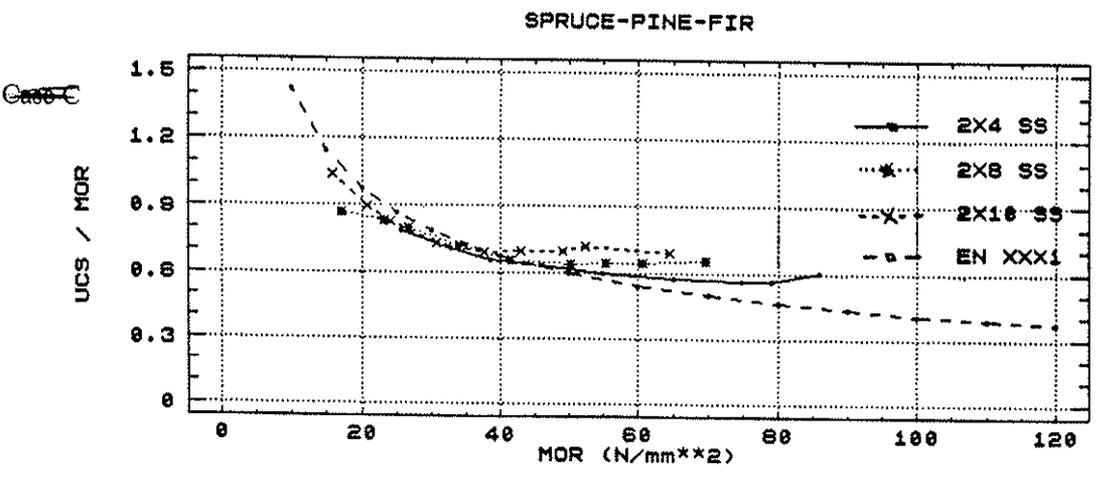
Figure 3. Compression/Bending Property Ratios for D Fir-L, Hem-Fir and S-P-F, Select Structural Grade.
