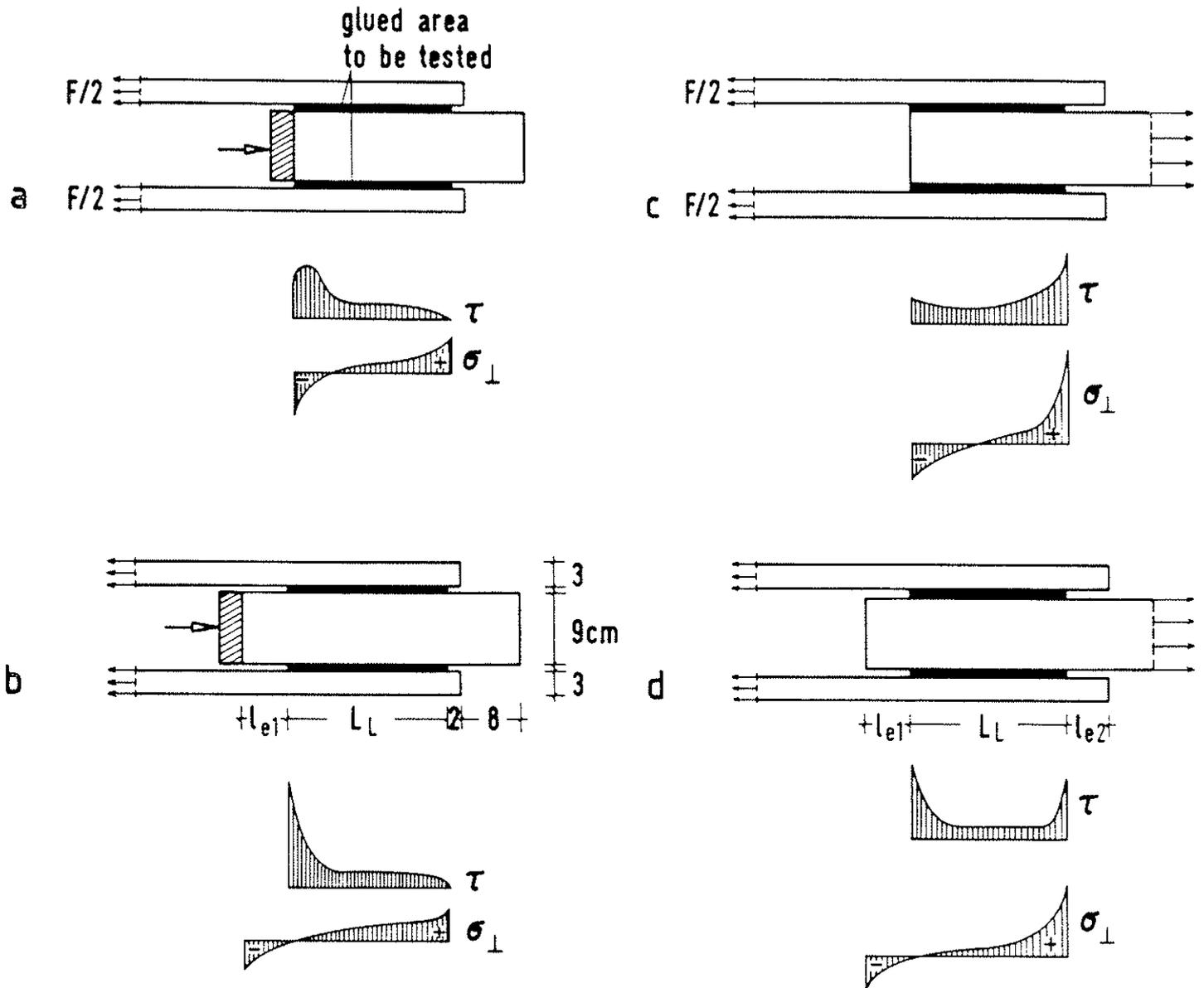
Figure 3: Specimens tested and stress distribution along the glue line in relation to load transmission mode and end distance
