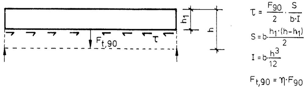
Fig. 5: Actions on the beam with depth  $h_1$ , separated from the beam with total depth  $h$ .
