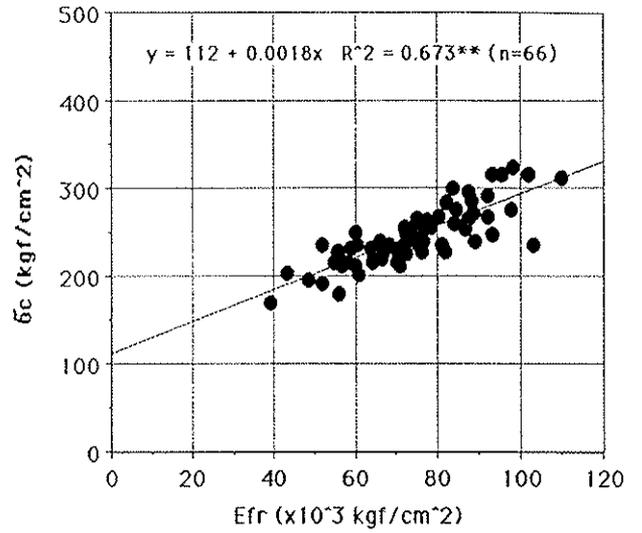
Figure 2. Relationship between Efr and compressive strength ( $\sigma_c$ )
