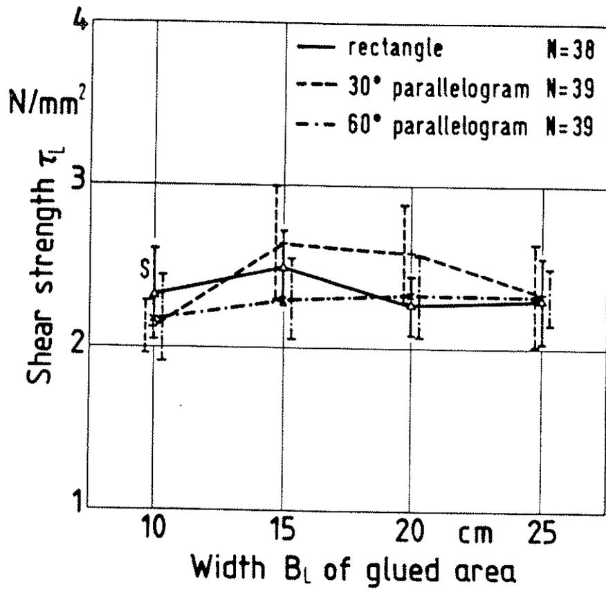
Figure 7: Effect of width  $B_L$  of glued area on shear strength  $\tau_L$  ( $l_{e1} = 5$  cm,  $\alpha = 0^\circ$ ,  $L_L = 20$  cm)
