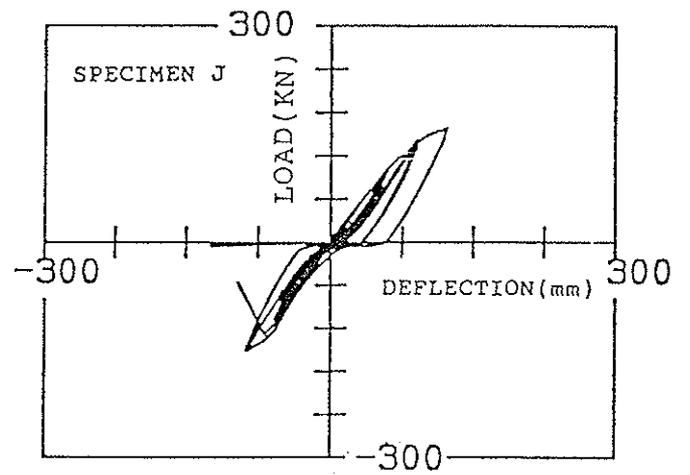
Fig.5 LOAD-DEFLECTION CURVES OF EACH SPECIMEN
