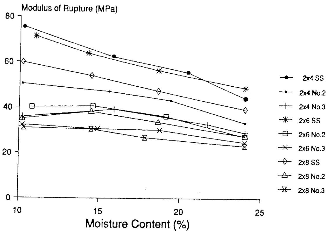
Figure 2: Relationships between the mean modulus of rupture and moisture content for Douglas-fir ( $M_p = 24$ ) (Aplin *et al* 1986)
