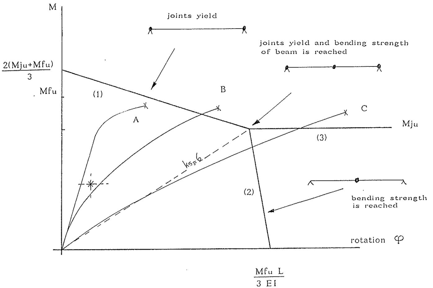
fig.3 : Requirements for rotation capacity
