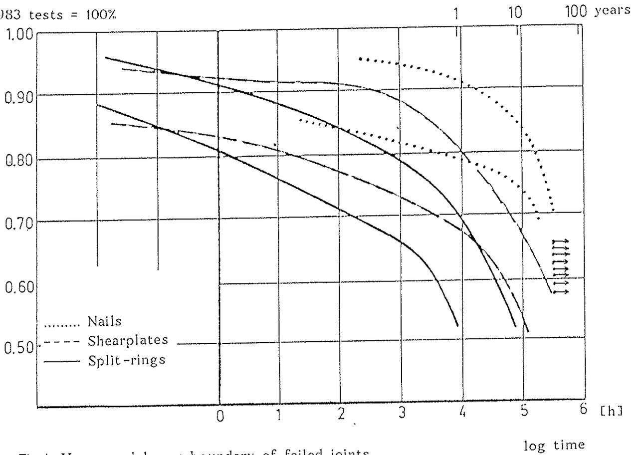
Fig.1: Upper and lower boundary of failed joints
