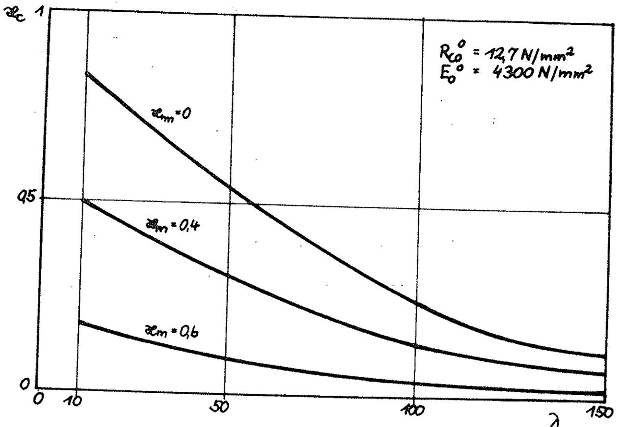
Figure 3: Dependence of  $\chi_c$  on  $\lambda$  for different  $\alpha_m$  ( $k_M = 0$ )
