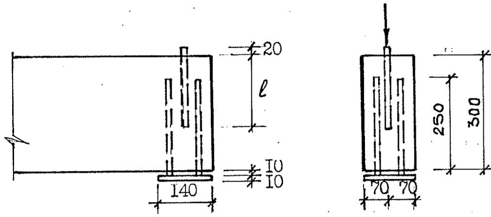
Fig. 1. Specimens of joints on steel bars glued-in across wood grain.
