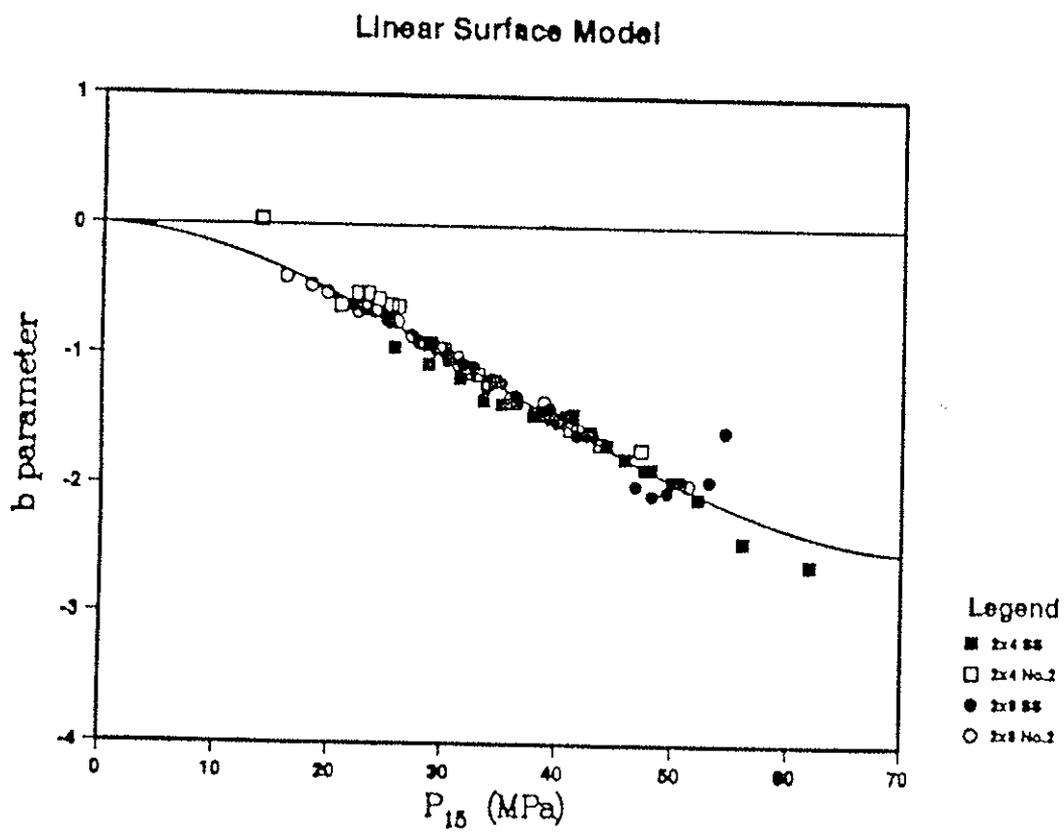
Figure 12: Relationship between the  $b$  parameter and  $P_{15}$  for 3-Term Linear Surface Model and showing the cubic regression fit to Douglas-fir compression strength data
