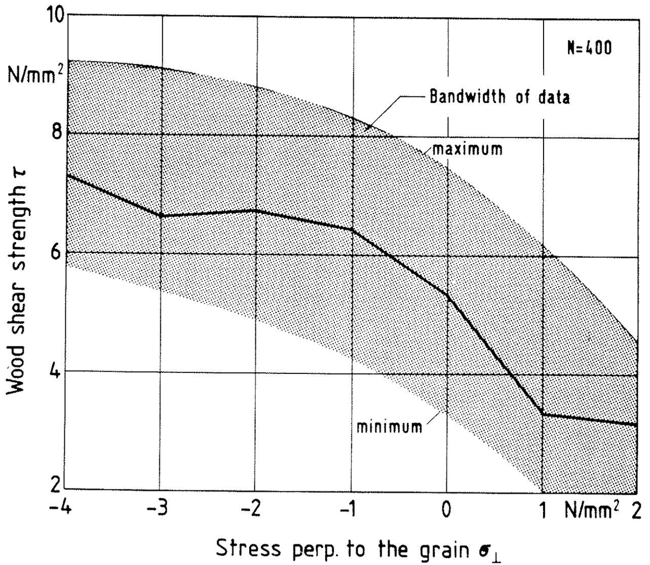
Figure 5: Effect of stress perpendicular to the grain on wood shear strength. According to Spengler (1982).
