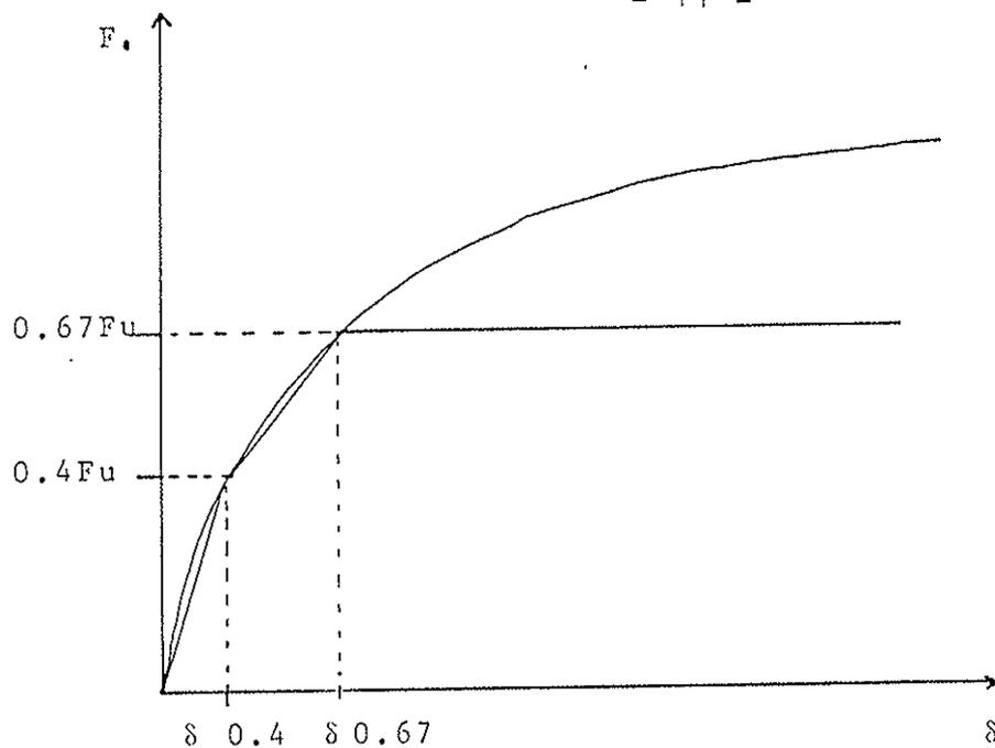
fig.6: Linear schematisation of the load slip curve of steel reinforced joints.
