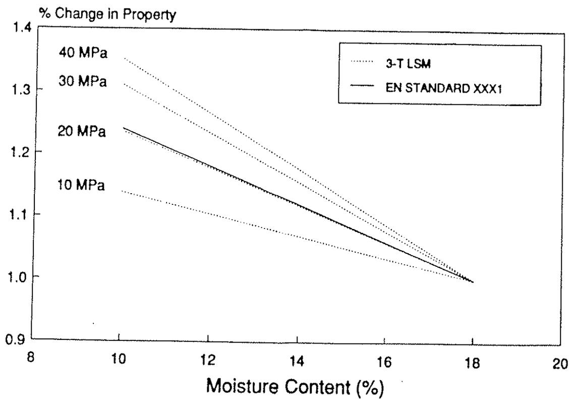
Figure 21: Comparison between CEN recommendations and 3-term compression strength linear surface model
