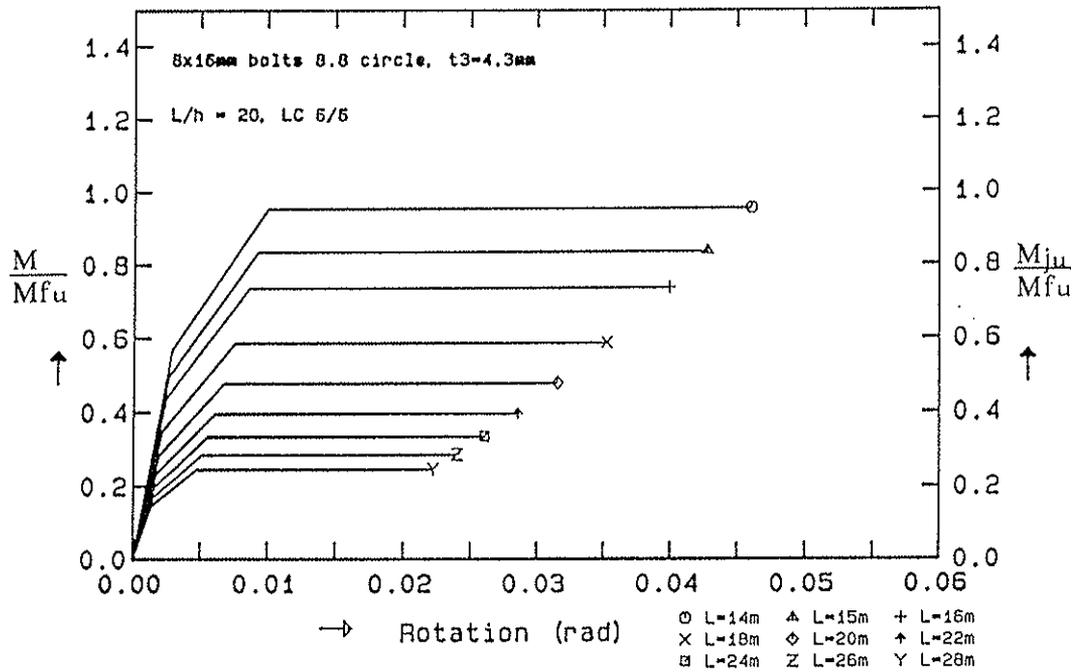
fig.8: Moment rotation curves of a steel reinforced joint with a circle pattern
