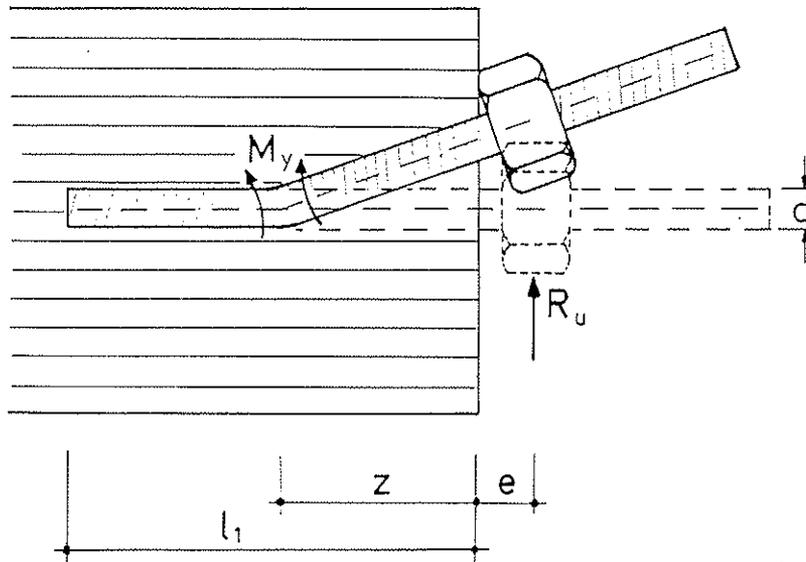
Fig.2: Schematic plot of the joint at ultimate limit state (failure mode)
