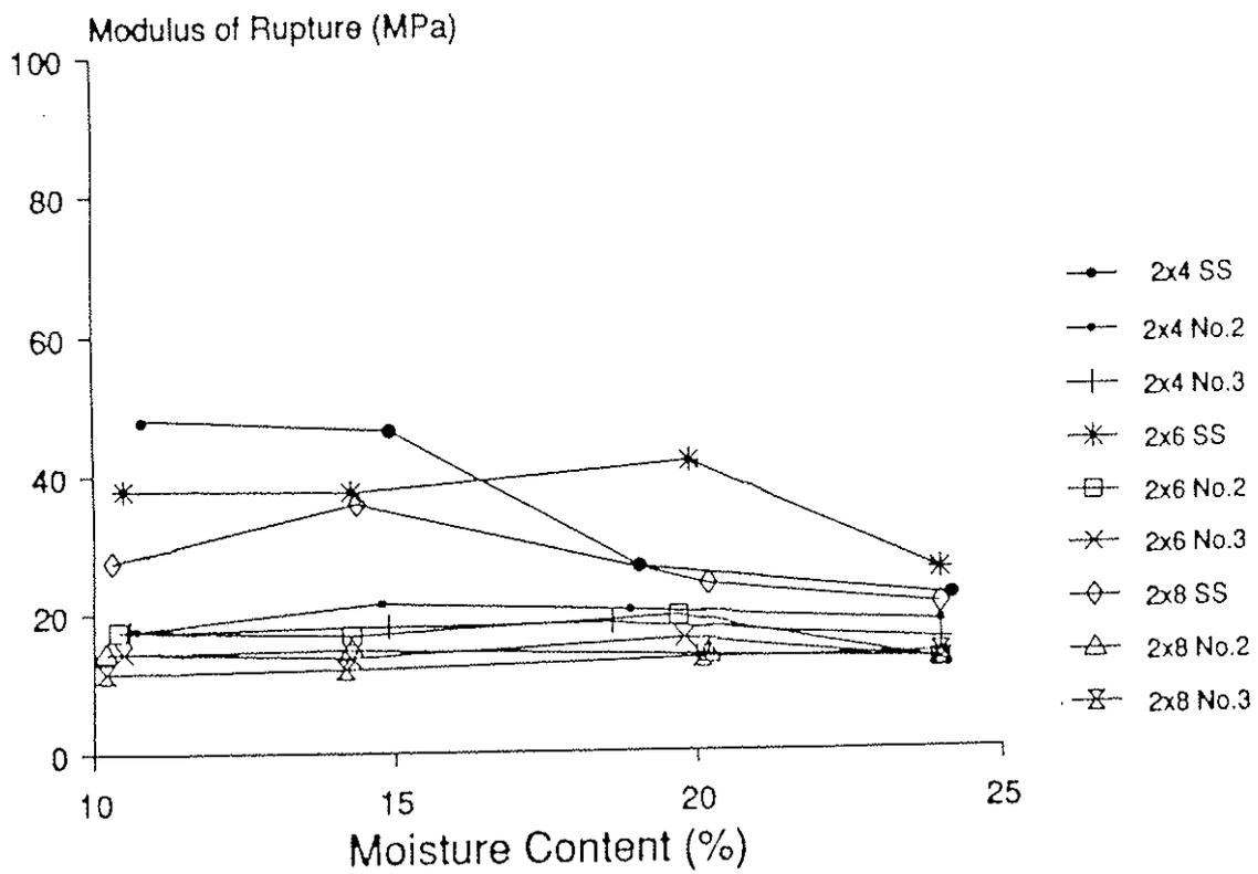
Figure 4: Relationships between the mean percentile modulus of rupture and moisture content for southern pine ( $M_p = 24$ ) (McLain *et al* 1984)
