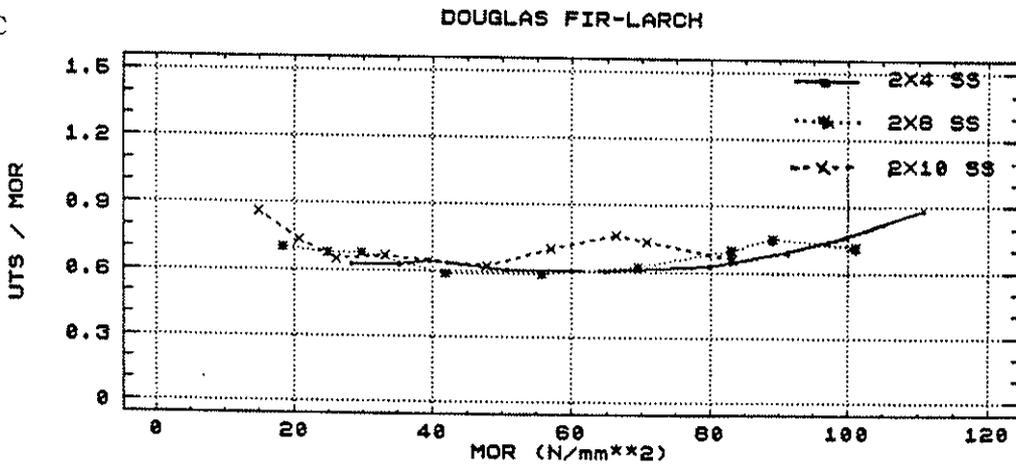
Figure 9. Tension/Bending Property Ratios for Case A, B, C Test Configurations - D Fir-L, Select Structural Grade.
