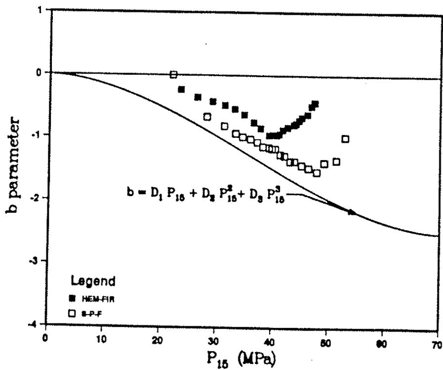
Figure 17: Relationship between normalized  $P_{15}$  and the  $b$  parameter for Hem-fir and Spruce-Pine-Fir Species (Compression Strength)
