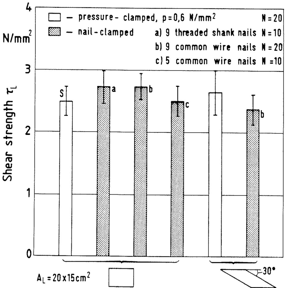
Figure 10: Effect of pressure technique on shear strength  $\tau_L$
