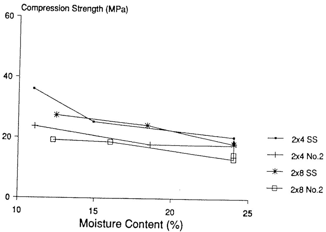
Figure 6: Relationships between the mean compression strength and moisture content for Douglas-fir ( $M_p = 24$ )
