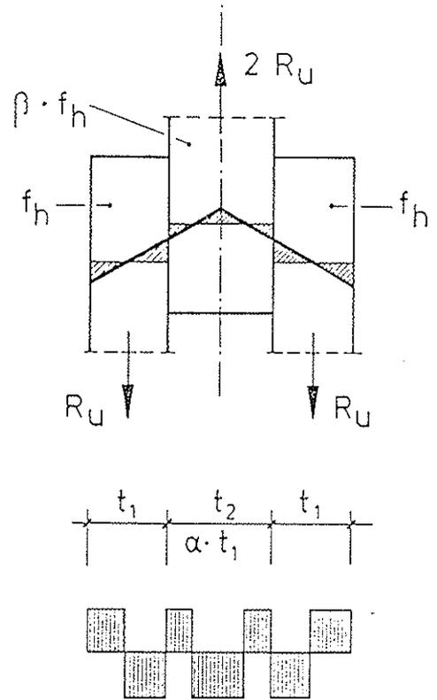
b) static model of the failure mode
