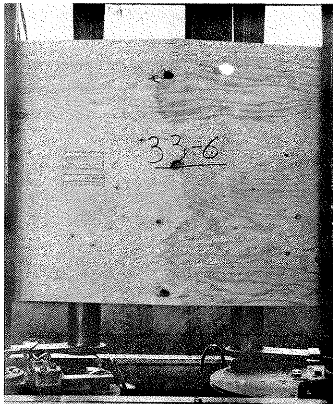
PLATE 1 PURE MOMENT FLEXURE TEST
