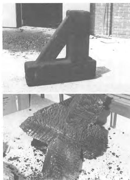
For the modern building fire escapes were required, which were added as external towers. Fire tests were carried out to determine the rate of charring and to determine what the effect there would be on the traditional joints.
