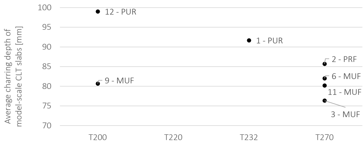
Figure 11. Charring depths of model-scale CLT slabs classified according to the classification system proposed in FprEN 18070.
