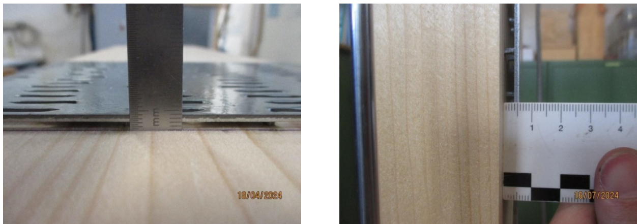
Figure 2.1. Test specimen with constant air gaps t_{air} \approx 2 \text{ mm} (left) and t_{air} \approx 4 \text{ mm} (right).
