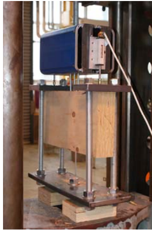
Figure 5. Direct Withdrawal Testing Apparatus for Screws in LVL
