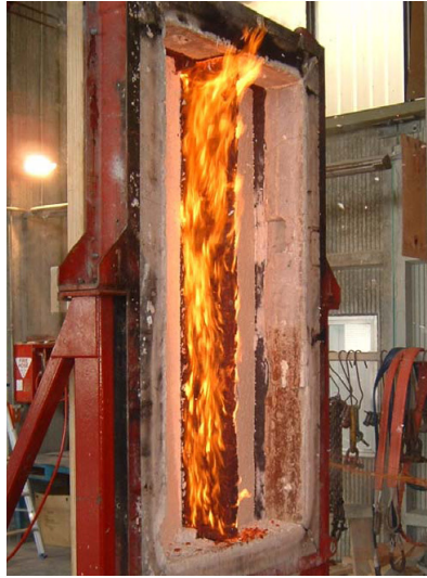
Figure 6: LVL beam in the pilot furnace during a test [13].
