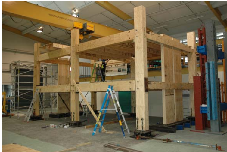
Figure 1. 2/3 Scale Post-Tensioned Test Structure at the University of Canterbury
