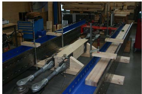
Figure 5: Test set-up for (a) single-row tests and (b) multiple-row tests
