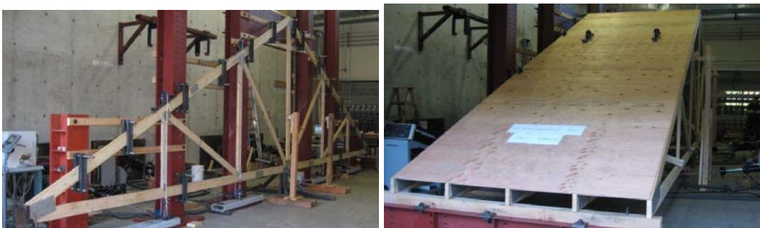
Fig. 3 Test setup for individual trusses and truss assemblies
