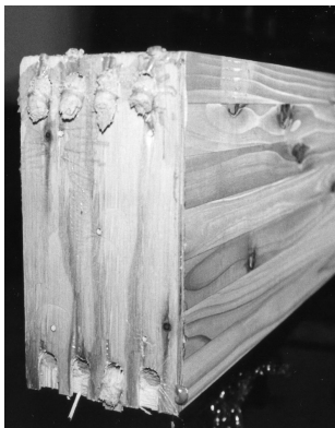
Fig. 11 Shear reinforced C4 specimen after testing
