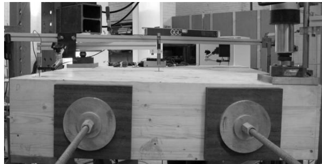
Figure 7 Test of "0° plate" with deflection measured in middle and in three corners.
