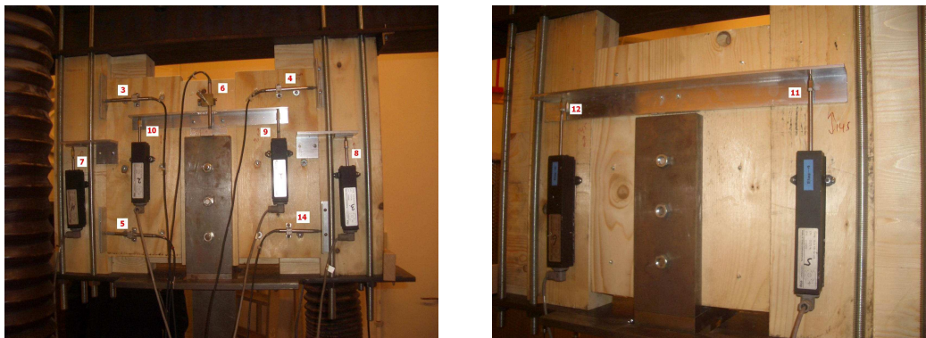
Fig. 3: Test specimen in front and rear view with instrumentation channels
