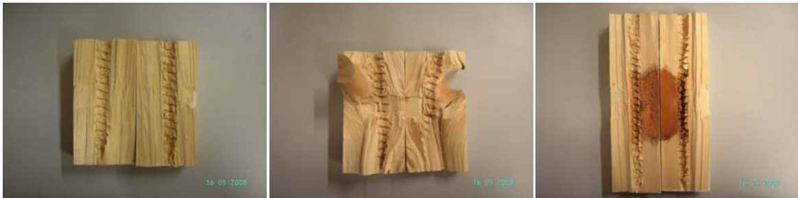
Figure 4: Selected small scale density and moisture specimens with clear wood, a knot and a resin inclusion
