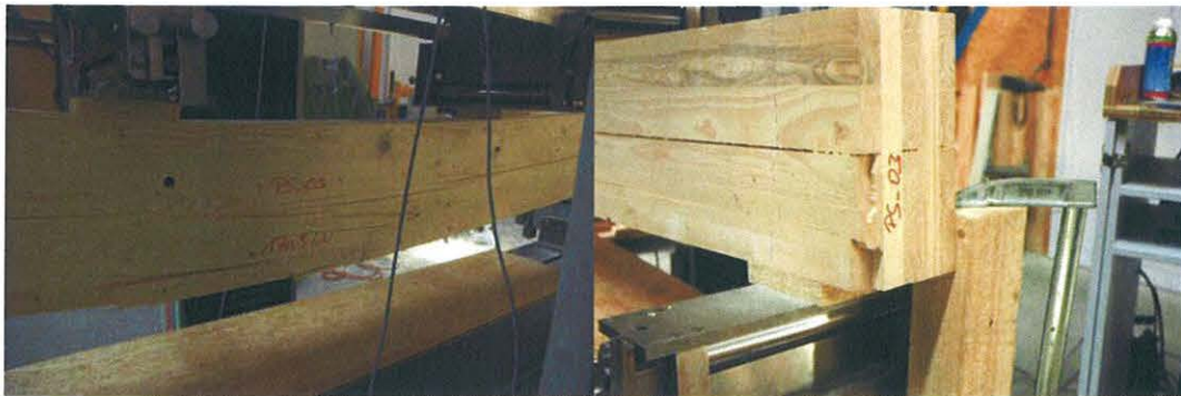
Fig. 9 Tensile failure in bending zone with local shear failure in tensile lamella in area of glue line.
