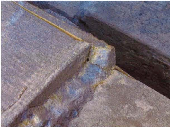
figure 4: Plastic deformation of timber fibre at the groove edge (Series K)
