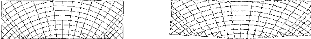
Figure 3.4: FE-net and deformed shape of the lamination
