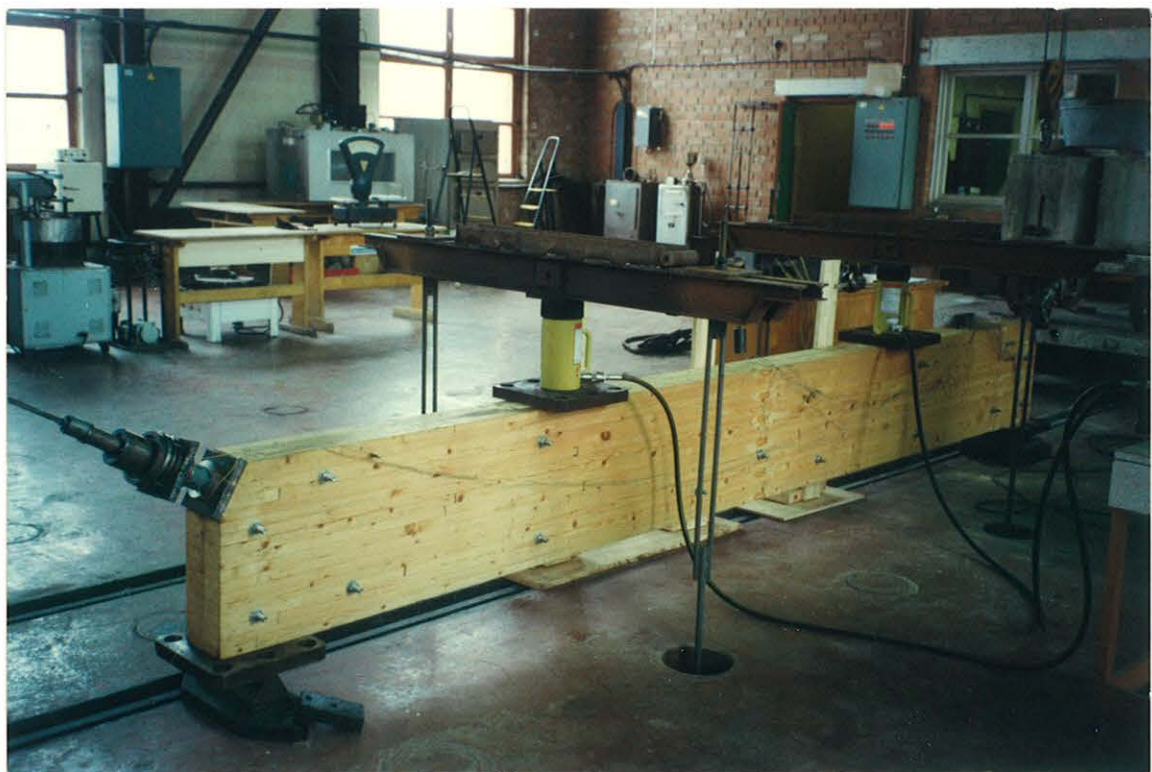
Figure 2. Loading of the prestressed glulam beam - model 6.
