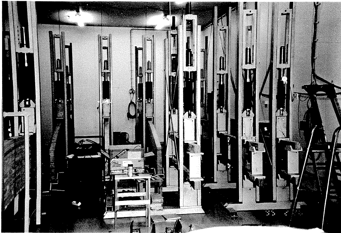
Upper Photo (n° 5) : short term test of curved beams in Lab 2
