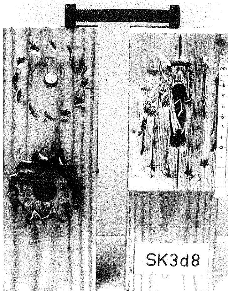
Fig. 1: Typical failure of a Bulldog tooth-plate connection
