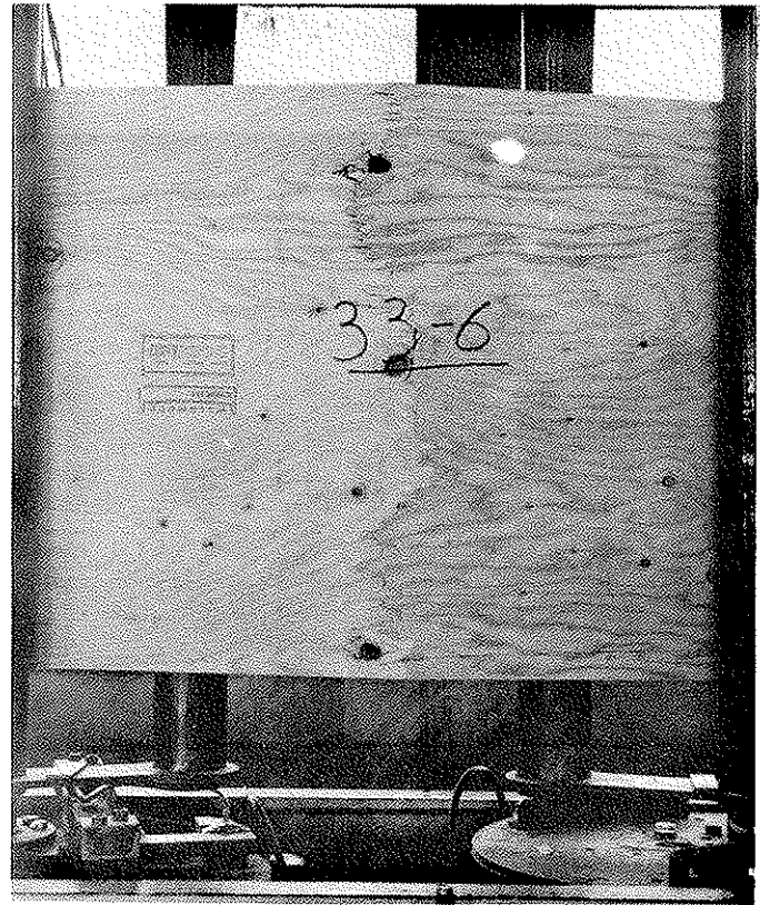
PLATE 1 PURE MOMENT FLEXURE TEST
