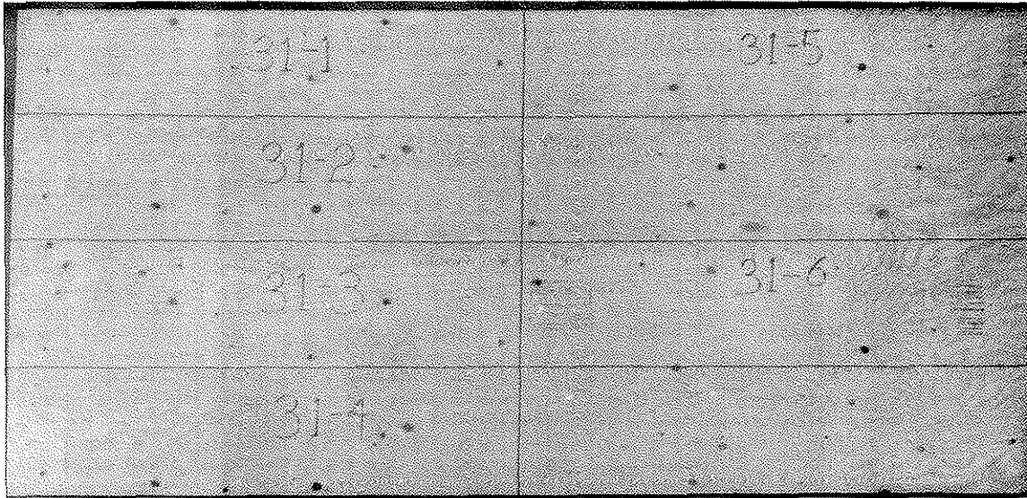
PLATE 3 TYPICAL SPECIMENS IN AN IN-GRADE PLYWOOD PANEL BEFORE CUTTING
