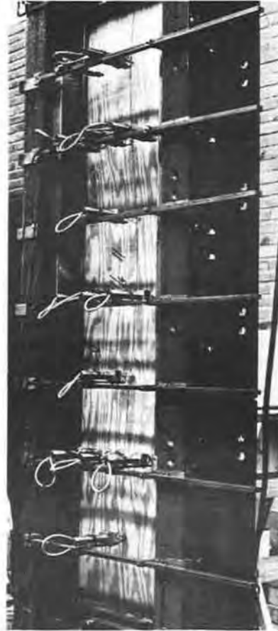
Simply supported test specimen, loaded parallel to direction of face grain. \beta = 4 ; 3 halfwaves.
