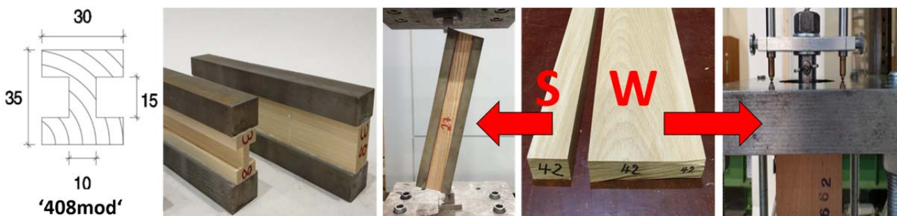
Figure 3. Shear (S) tests and withdrawal (W) tests performed on the same raw material.
