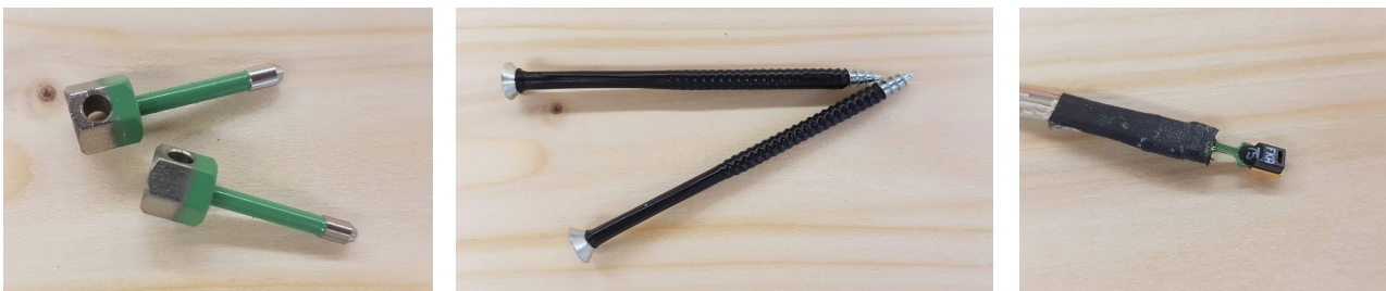
Figure 2: Partially Teflon coated GANN electrodes (left), partially insulated screws (middle) and CMOS relative humidity and temperature sensor (right).
