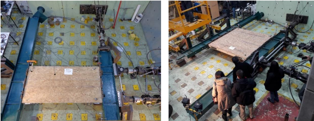
Figure 2. Shear walls tests specimens subjected to cyclic shear plus gravity load and overturning moment action.
