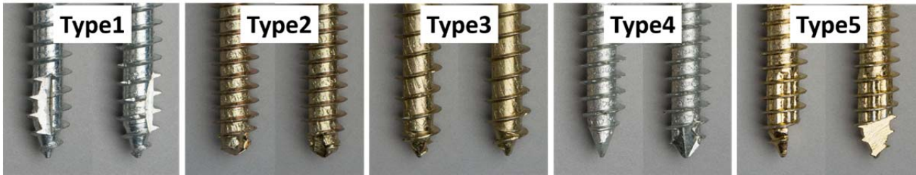
Figure 12. Tip shapes of the five different screw types applied in this part of the study.
