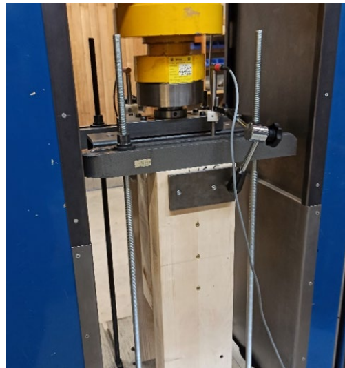
Figure 5. Test setup for |-| type CLT/CLT/CLT connection for cyclic testing in compression and tension.
