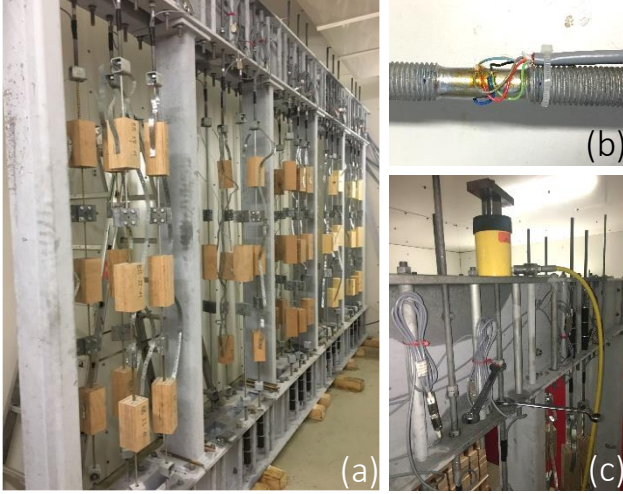
Figure 3.1. (a) DoL test frame; (b) strain gauges; (c) uploading via hydraulic cylinder and manually.
