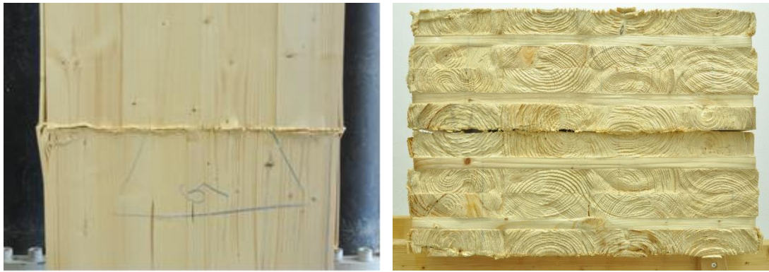
Figure 1: Typical compression failure at end grain contact joint in CLT: joint after failure (left), contact surfaces with mutual imprints of annual rings (right)
