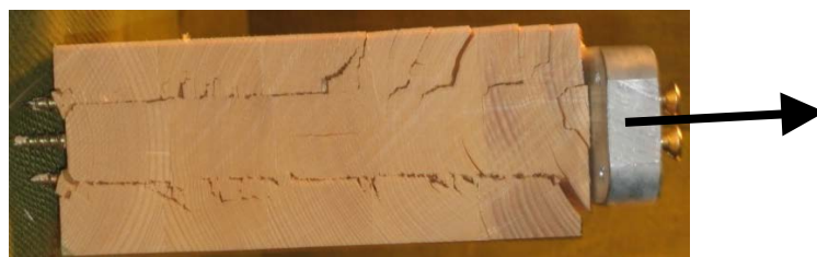
Fig. 3: Block shear failure (mode (c) in Figure 1) with rolling shear failure over the complete beam depth caused by axially loaded screws perpendicular to grain in glulam.
