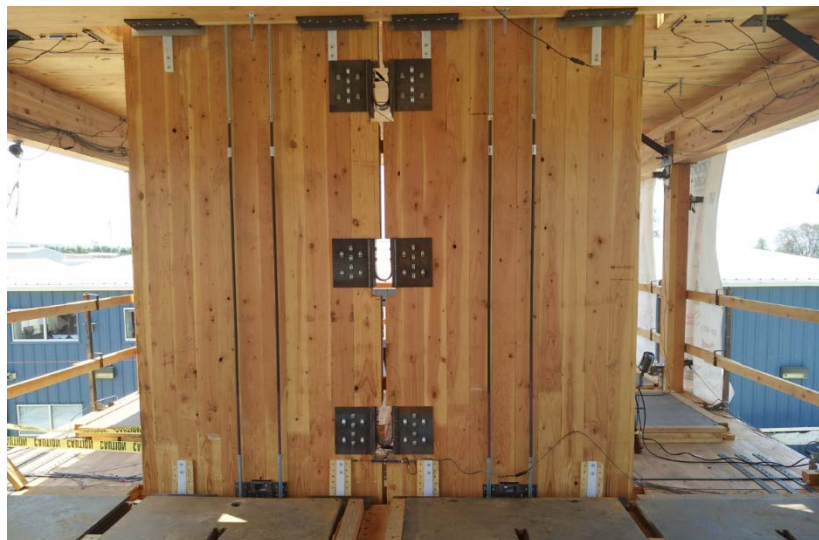
Figure 3: Post-tensioned CLT rocking walls coupled with UFP connectors and attached to the CLT diaphragm with shear-transfer-only connectors (viewed from the 2 nd floor)
