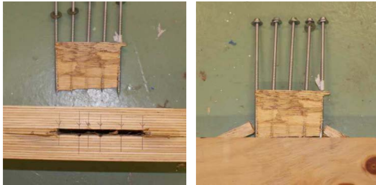
Figure 2: Row shear failure (mode (d) in Figure 1) in connections with axially loaded screws perpendicular to grain in LVL from Carradine et al. 2009 [2].
