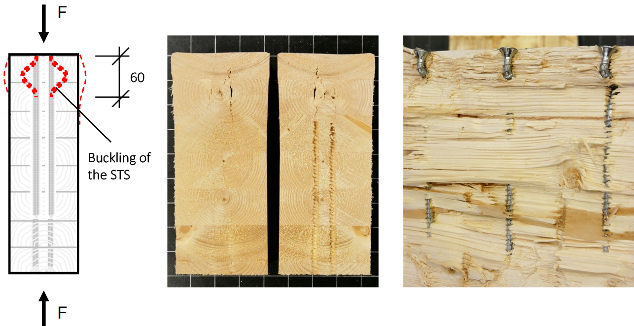
Figure 12. Sketch of deformation behaviour (left), lateral extension of specimen below the contact plate (middle), buckling of STS perpendicular to the grain (right).
