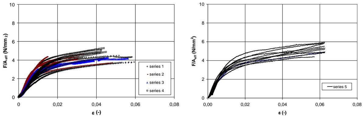
Figure 4: Stress-strain-diagrams for support loading (case 4).
