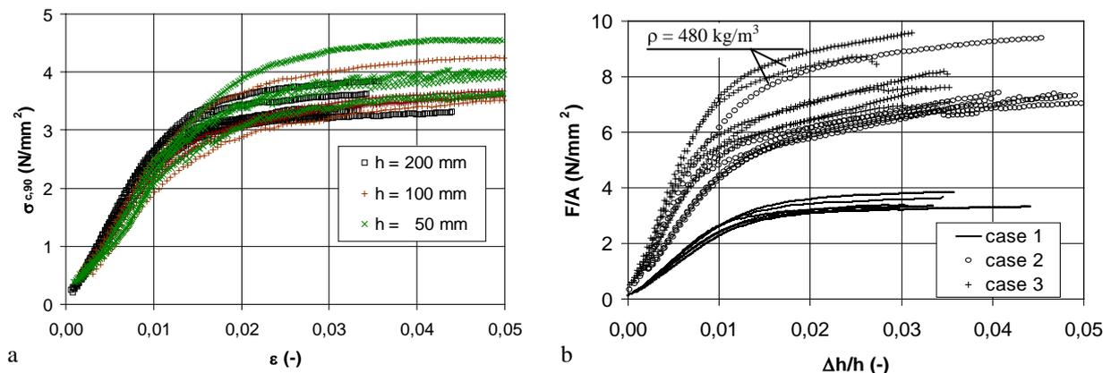
Figure 2: Stress-strain-diagrams, a) Case 1,  $h = 50, 100$  and  $200 \text{ mm}$
