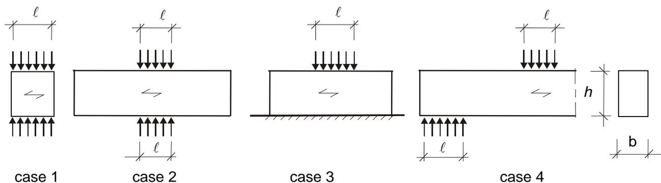
Figure 1: Different loading situations in compression perpendicular to the grain
