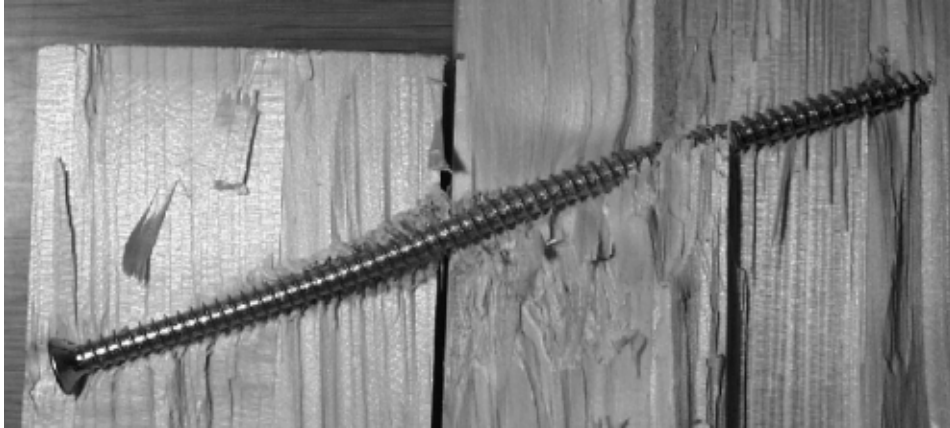
Figure 4: Sliced specimen with self-tapping screw
