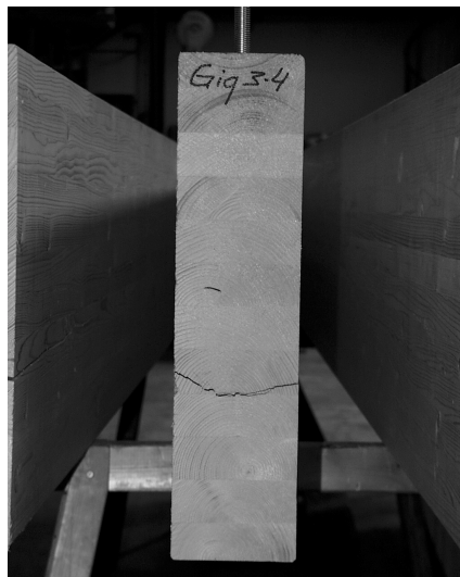
Figure 2: Tensile failure perpendicular to the grain
