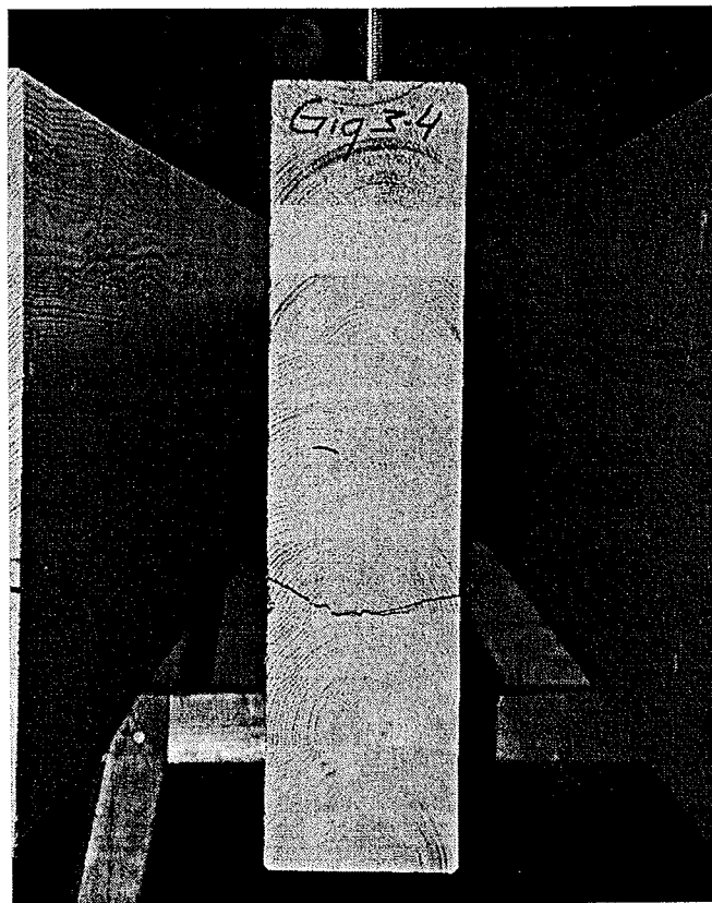
Figure 17: Tensile failure perpendicular to the grain
