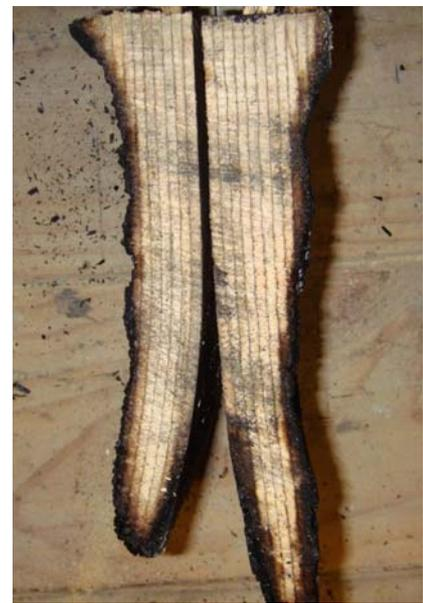
**Figure 3: Residual Section of the 400 mm Floor**
