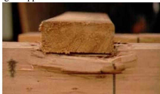
Figure 5: Plastic failure mode
